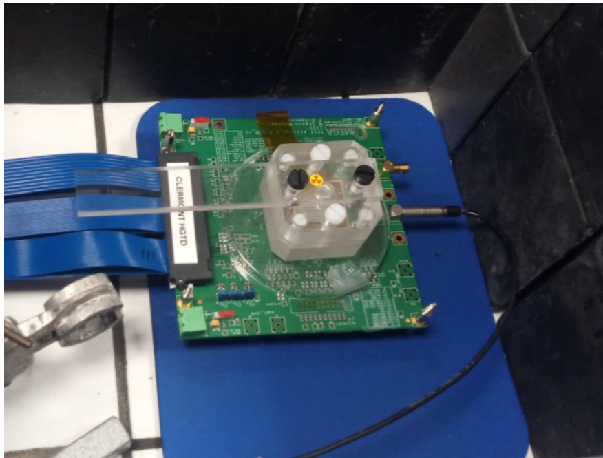
Figure 5.19: Strontium \text{Sr}^{90} placed on top of the LGAD bump-bonded on ALTIROC2.
