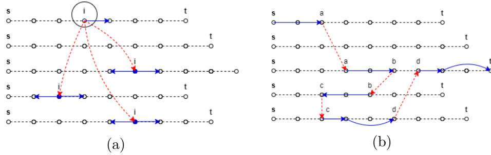
Figure 5.2 – (a) Possible actions (jump in red, direction in blue) given the last visited customer i ; (b) a possible sequence generated with 4 jumps (in red) given a pool of 5 sequences of visits
