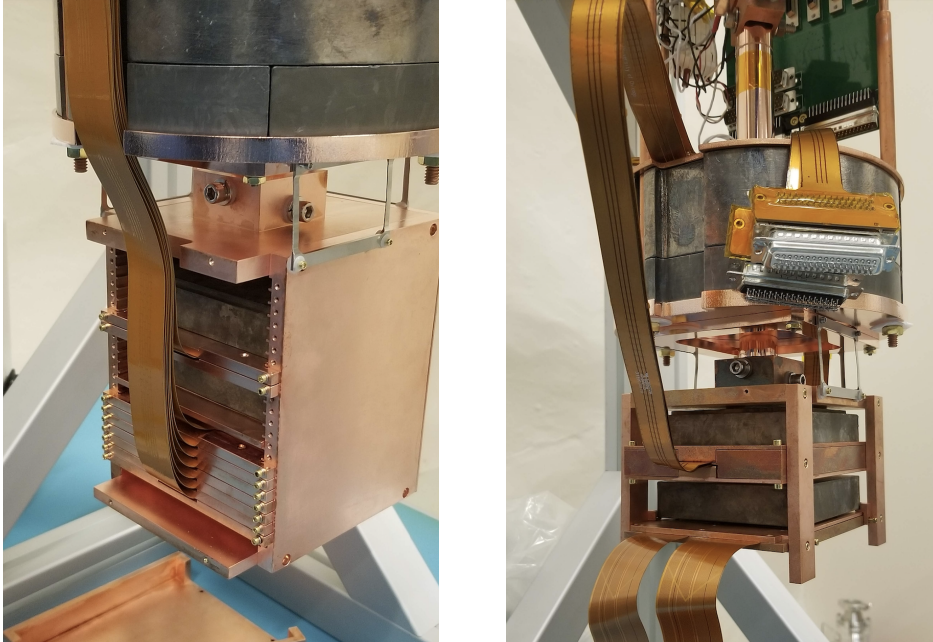
Figure 3.2: DAMIC detector at SNOLAB before (left) and after (right) the upgrade of 2021. Left: Tower of 8 CCDs (36 g target mass). Right: DAMIC and SENSEI new skipper CCDs.
