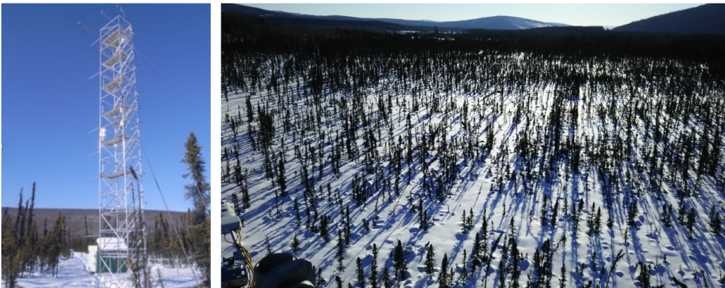
Figure 4.5: Left: photo of the 17 m high measurement tower at the Poker Flats Research Range Ameriflux site. Right: photo of the PRR site as seen from the measurement tower. Credit: Lisa Johnson.
