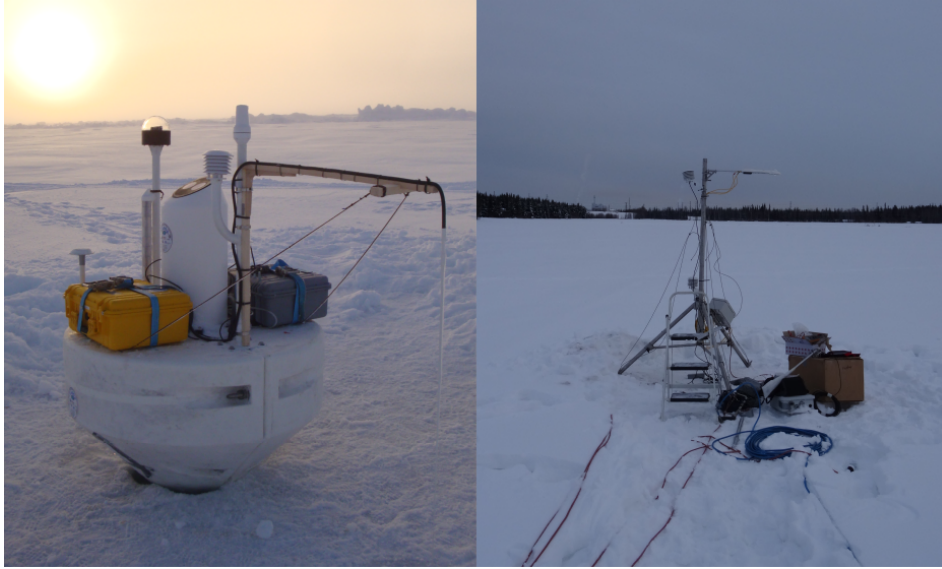
Figure 1.11: Left: photo of a IAOOS buoy locked into the ice in the Arctic Ocean. The lidar is the white tube and temperature sensors are located on the mast. Photo taken by V. Mariage [Mariage 2015]. Right: photo of the measurement mast during the pre-ALPACA campaign in Fairbanks, Alaska. The CNR4 radiometer is visible; the sonic anemometer hadn't yet been installed. Photo taken by J. Maillard.
