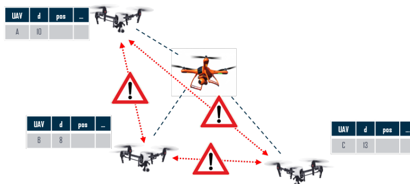
Figure 5.16 – Detection of a target, construction of an internal table for each UAV, and appearance of potential local communications vulnerabilities.
