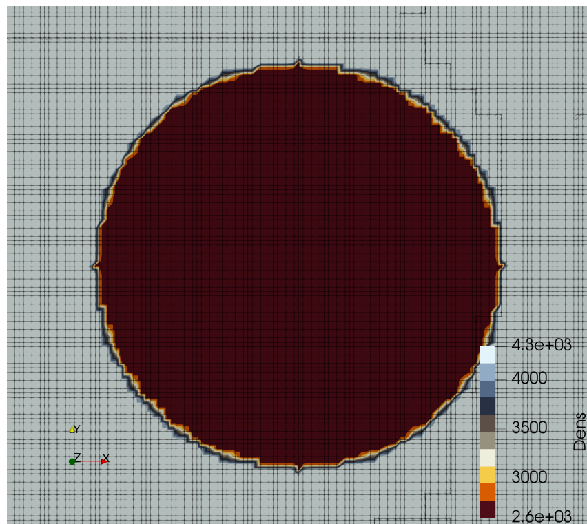
Figure A.4: Density distribution using the non honouring technique for a semi-spherical basin model observed at the surface. The mesh is discretized at the GLL points described by a non regular distance.
