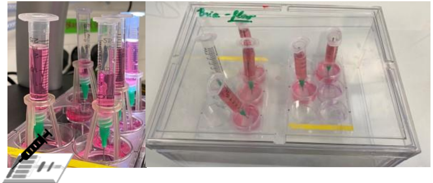
Figure 2.12: Using a gravity driven perfusion allow to run multiple experiments in parallel with a simple setup Using syringes as reservoirs, we can apply a gravity driven perfusion method to our chip. Making a unique input per chip allows to run multiple experiments in parallel. A picture of a typical setup is shown above
