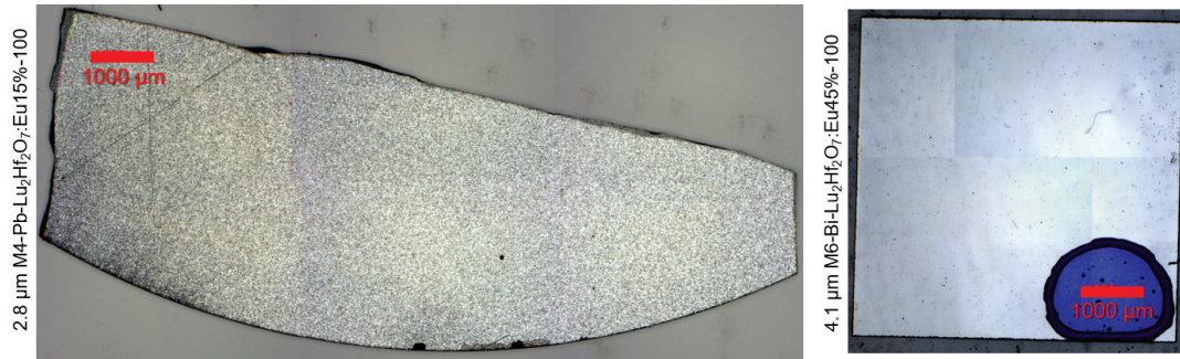
FIGURE 3.9: Micrographs of M4-Pb-Lu 2 Hf 2 O 7 :Eu15%-100 and M6-Bi-Lu 2 Hf 2 O 7 :Eu45%-100. Both have been lapped and polished on one side as preparation for usage at the beamlines for imaging experiments.
