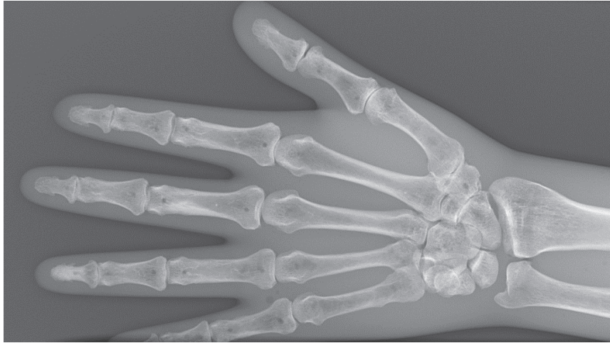
FIGURE 4.1: Radiograph of a hand, acquired with a 500 \mu\text{m} columnar CsI:Tl screen, adopted from [51].
