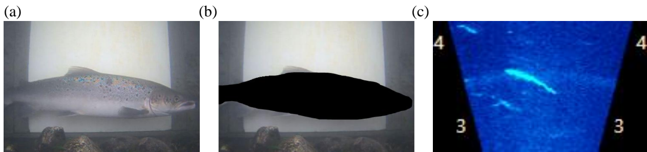
Figure 87 – Image of an Atlantic salmon captured by an optical camera at a fish way location © Fédération de pêche de la Somme (a) and the corresponding overall silhouette in black (b). Echo of an Atlantic salmon recorded on an ARIS 1800 image (c).
