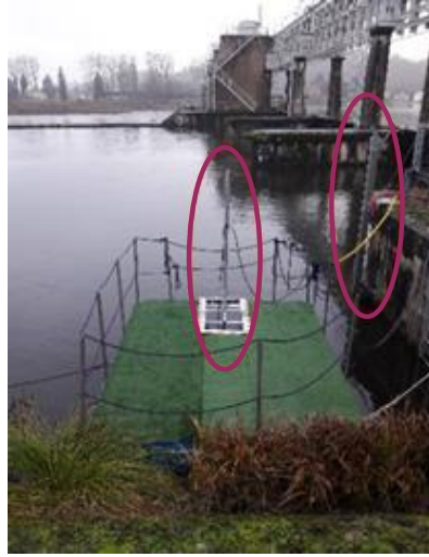
Figure 21 – Picture of the floating platform, on which the BlueView camera is fixed (left pink ellipse) and of the support of the ARIS 1800 (right pink ellipse).
