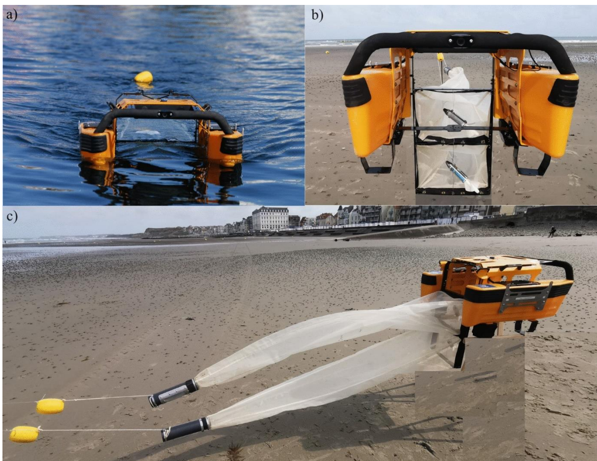
Figure 25 : Pictures of the aquatic drone innovative sampling device in different angles and configurations. a Aquatic drone during sampling, b aquatic drone equipped with double nets from the front, and c aquatic drone equipped with double nets from the side (each net having a dimension of 36 cm width, 25 cm height, and 200 cm length); each net is equipped with a flowmeter (General Oceanic®)
