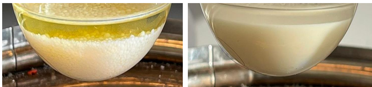
Figure V.4. Photographs of the mixture of the VP-SDPP@CCM-C latex with a [\text{Rh}(\text{COD})(\mu\text{-Cl})_2] /toluene solution ( P/\text{Rh} = 4:1 ) before (left) and after stirring (right).
