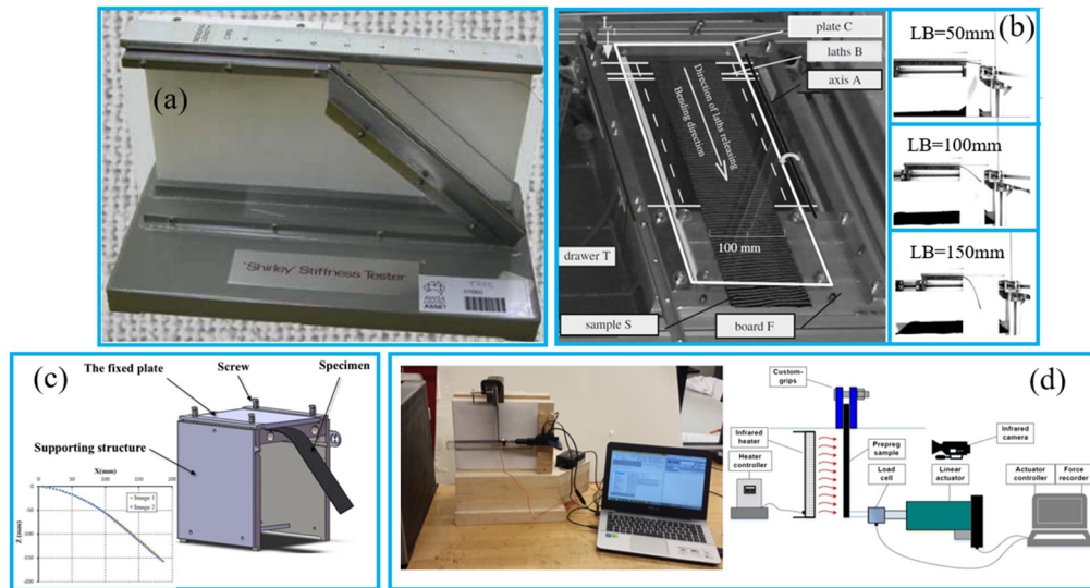
Fig. 1.16 The Peirce cantilever beam method, (a) standard cantilever bending test [94], (b) new flexometer-cantilever bending test fixture [102], (c) support for the high thickness specimen clamping [93] and (d) vertical cantilever bending test system [105].
