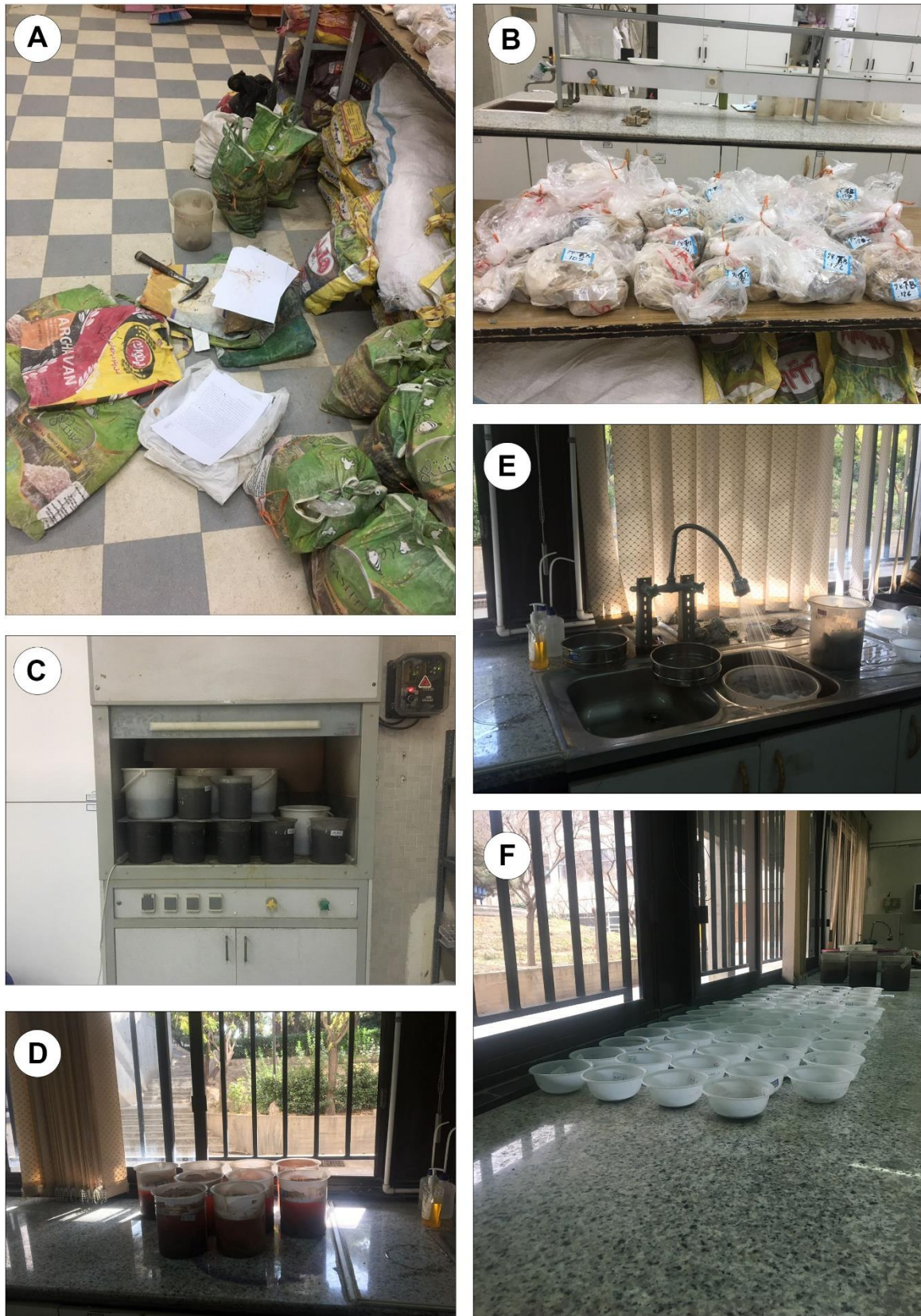
Fig. 3.7. Laboratory images showcasing the preparation of samples from the Ali-Bashi and Baghe-Vangh sections in Iran for conodont extraction, employing two distinct techniques (10% \text{CH}_2\text{O}_2 and 15% \text{CH}_3\text{COOH} ).
