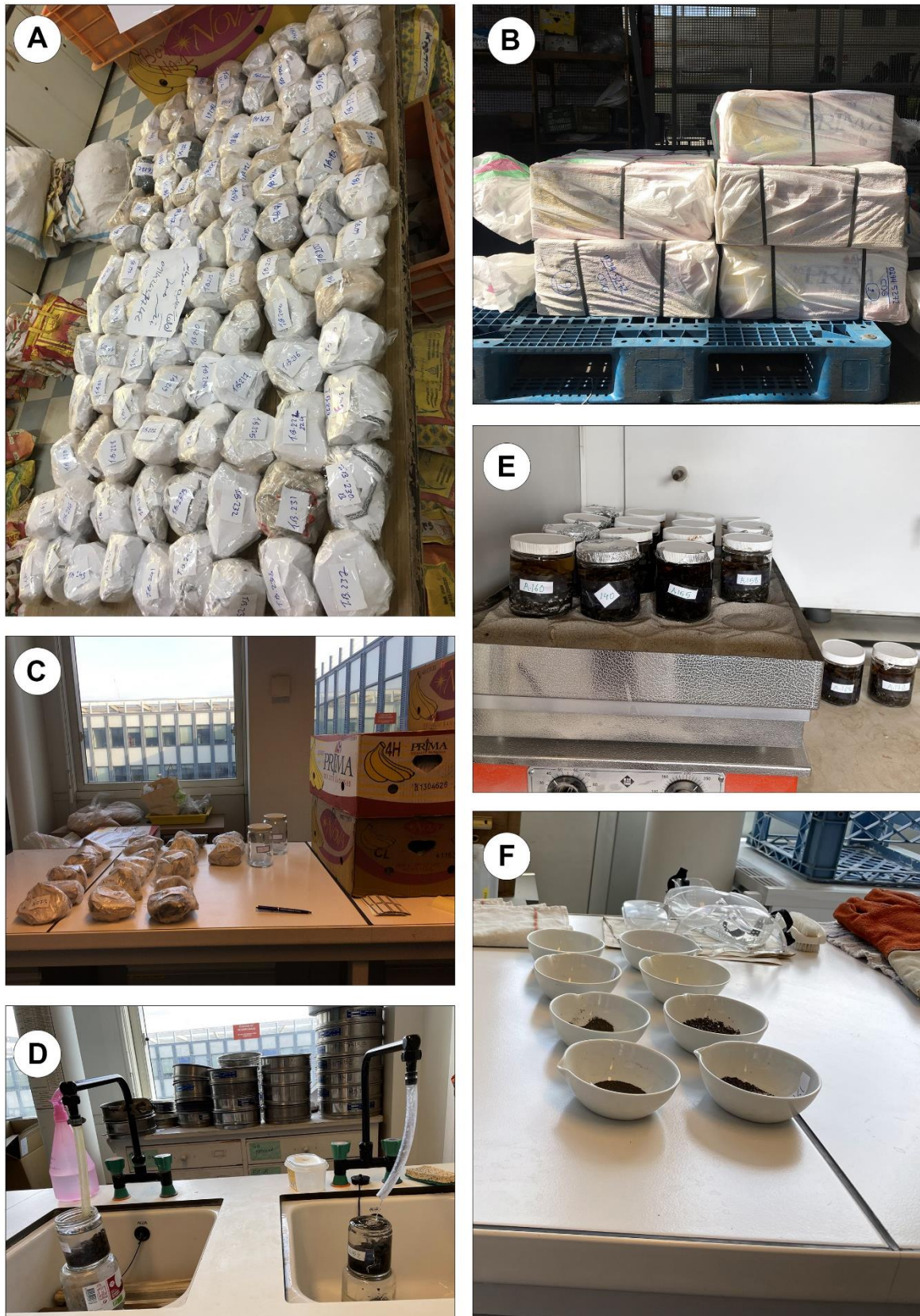
Fig. 3.9. Complete series of laboratory procedures conducted in CR2P, France, encompassing various stages such as sample transportation (A-B) and the subsequent preparation utilizing the hot acetolysis protocol according to Crasquin et al. (2005) (C-F).
