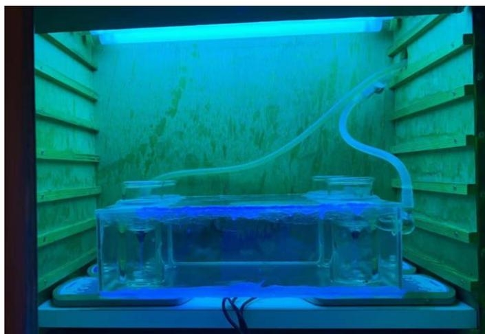
**Fig.V-2** Equipment for irradiation experiments.
