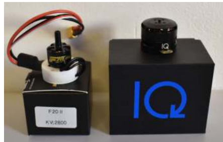
Figure 4.3.: Motors provided by Vertiq (former IQ-Motion). On the left, a F 20 II motor with a custom magnetic encoder, controller, and firmware installed by Vertiq. On the right, a Vertiq module.
