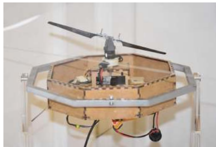
Figure 4.6.: First gimbal system used to test the swashplateless device. a) Unloaded. b) Loaded with a Pixhawk Mini 4 card controlling the Vertiq module.
