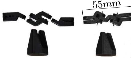
Figure 4.5.: Some 3D printed swashplateless assemblies. The one on the left was printed on an Ultimaker S5 using ABS plastic. The assembly on the right was printed on a Volumic MKII printer, using PLA plastic.
