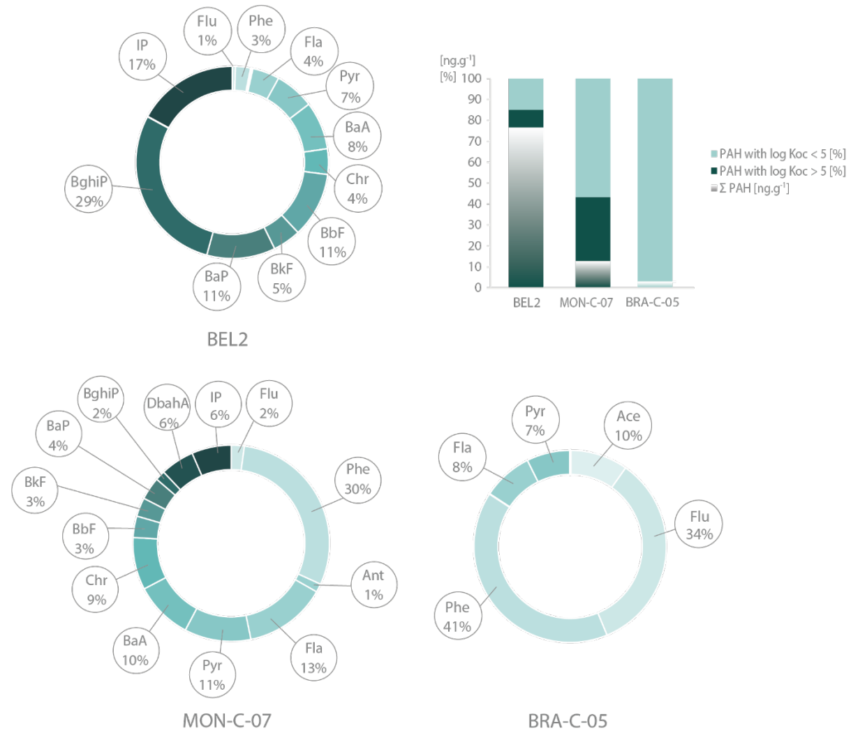
Figure 9-2. PAH results in the different USCDs. The circles indicate the proportion (%) of each PAH relative to the total PAH concentration. The top-left histogram indicates both the proportion (%) of hydrophilic PAHs (with \log K_{oc} < 5 , in light blue) and hydrophobic PAHs (with \log K_{oc} > 5 , in dark green), while the white limit corresponds to the total PAH concentration ( \text{ng.g}^{-1} ).
