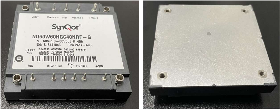
Figure 3.2. DC/DC converter module NQ60W60.
