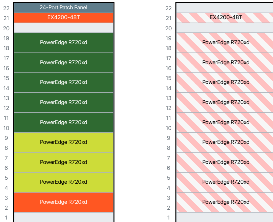
Figure V.5: NetBox model of a 22 U datacenter rack (front and rear of the rack)
