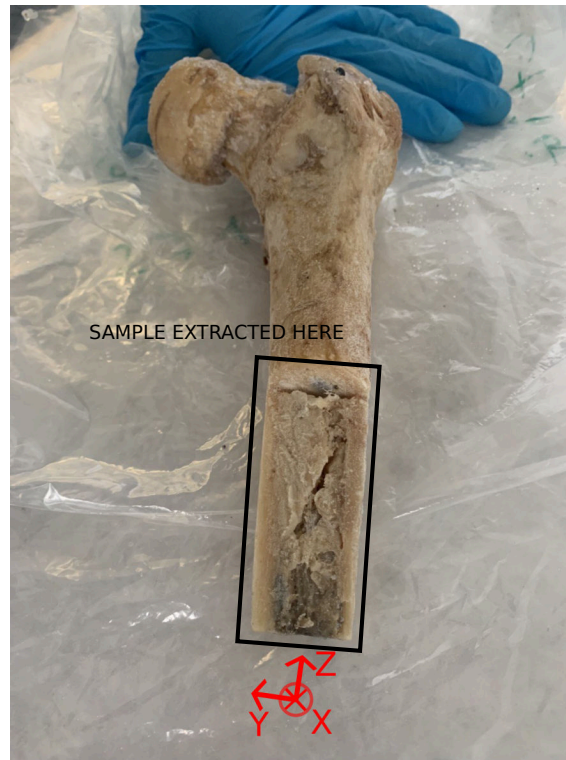
Figure 4.1: Extraction of half-cylinder bone samples from femoral shafts for analysis. Each sample, approximately 7 cm in length, was extracted along the femoral axis at the mid-diaphysis.
