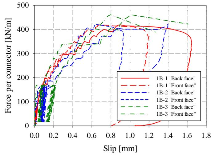
a. Force per connector versus slips
