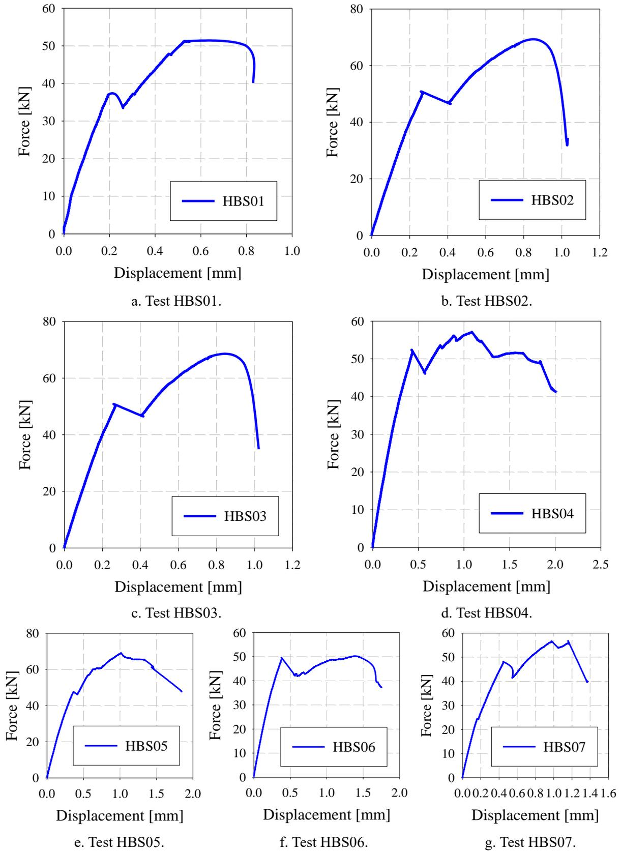
Figure 3: Force-displacement curves of rolling shear tests.
