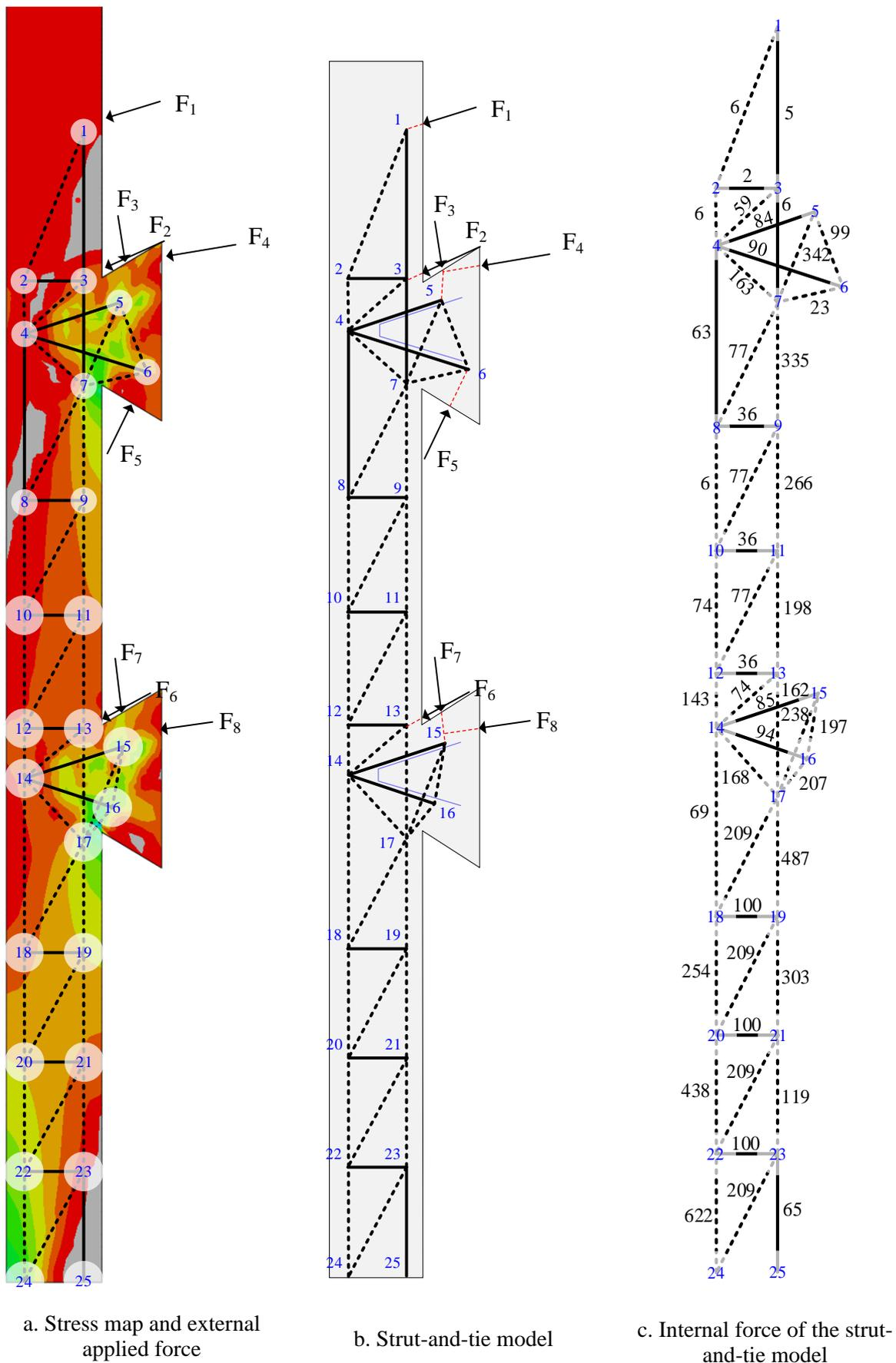
Figure 56: Proposed strut-and-tie model deduced from principal stress map of FE model and the obtained internal forces of the strut-and-tie model at yielding stress of rebars.
