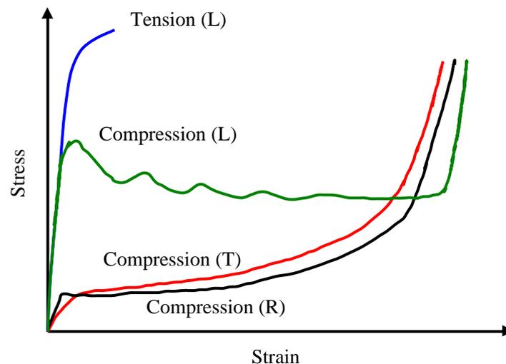
Figure 8: Typical stress-strain curves for timber [53].
