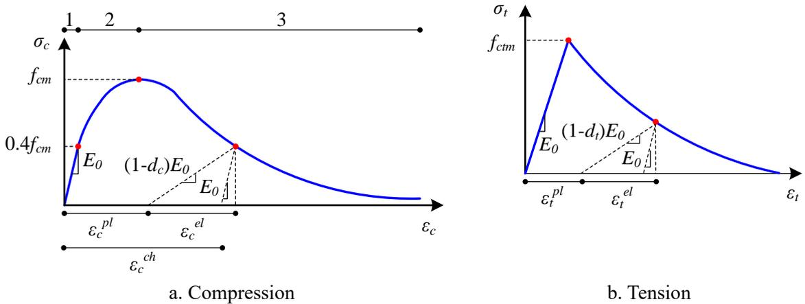
Figure 6: Stress-strain curves of concrete under uniaxial loading [46].
