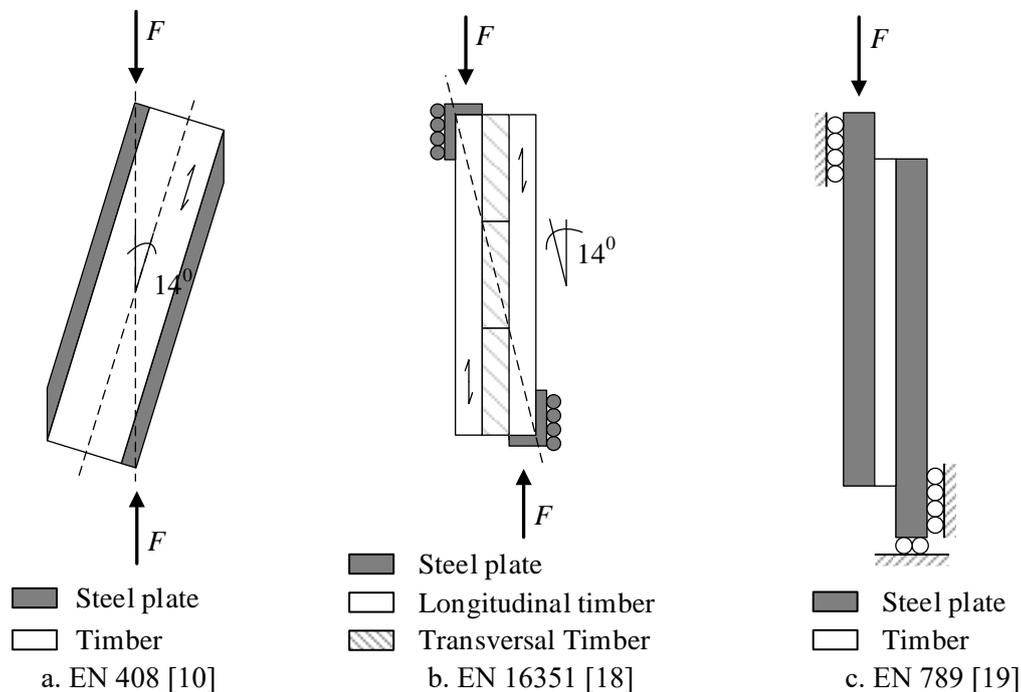
Figure 8: Direct shear test setups.
