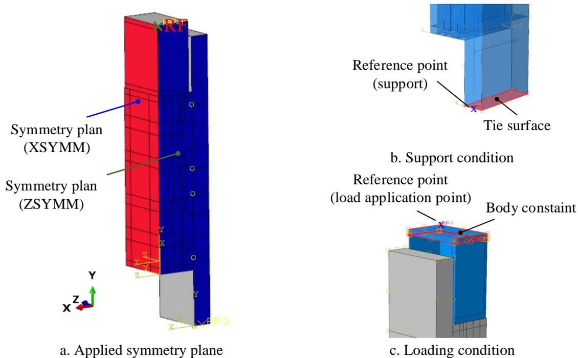
Figure 21: Boundary conditions, support condition, and loading of the pushout test in the finite element program.
