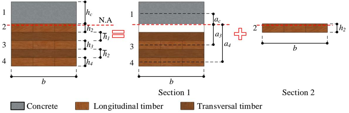
Figure 25: Computation of 5-layer CLT-concrete slabs [3].
