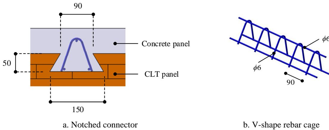
Figure 1: Dovetail-shape notched connector (unit in mm).
