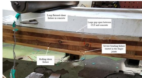
c. Typical failure mode in flexural tests
