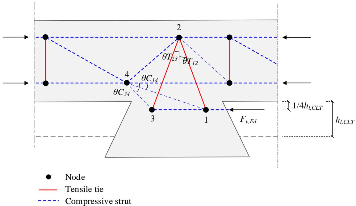
Figure 4: Strut-and-tie model of the concrete notch.
