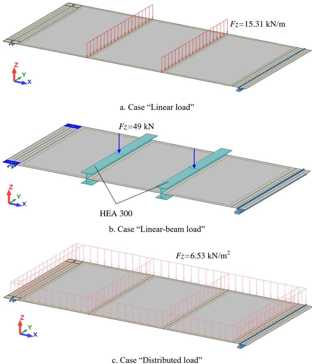
Figure 38: Loading configurations applied on the plate model.
