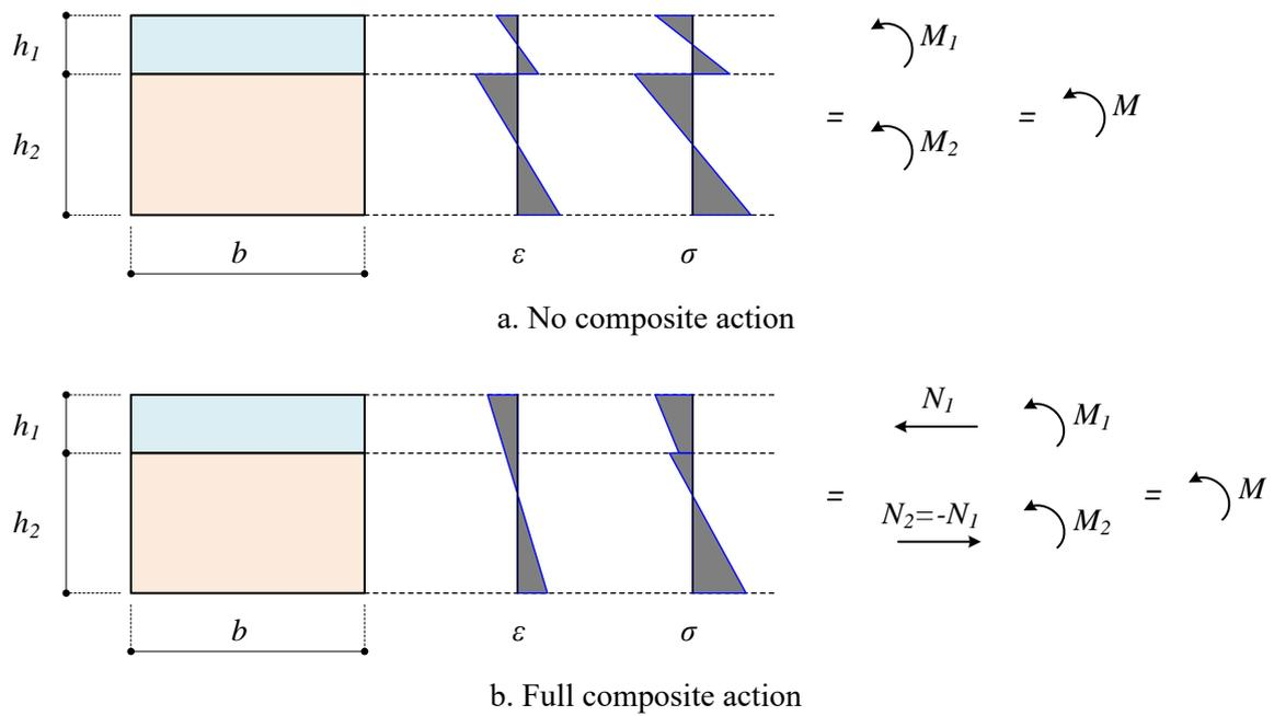
Figure 22: Strain distribution in the cross-sections of timber-concrete composite floors with different composite efficiencies.
