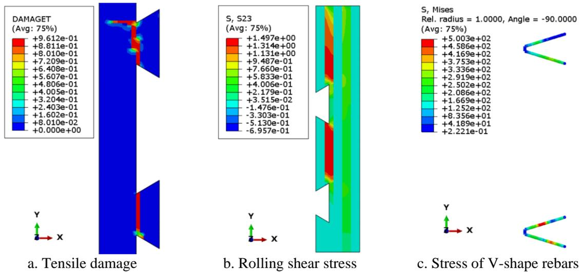
Figure 39: Tensile damage of the concrete panel, rolling shear stress of the CLT panel, and tensile stress of V-shape rebar in case C3-1 at a maximum load level.
