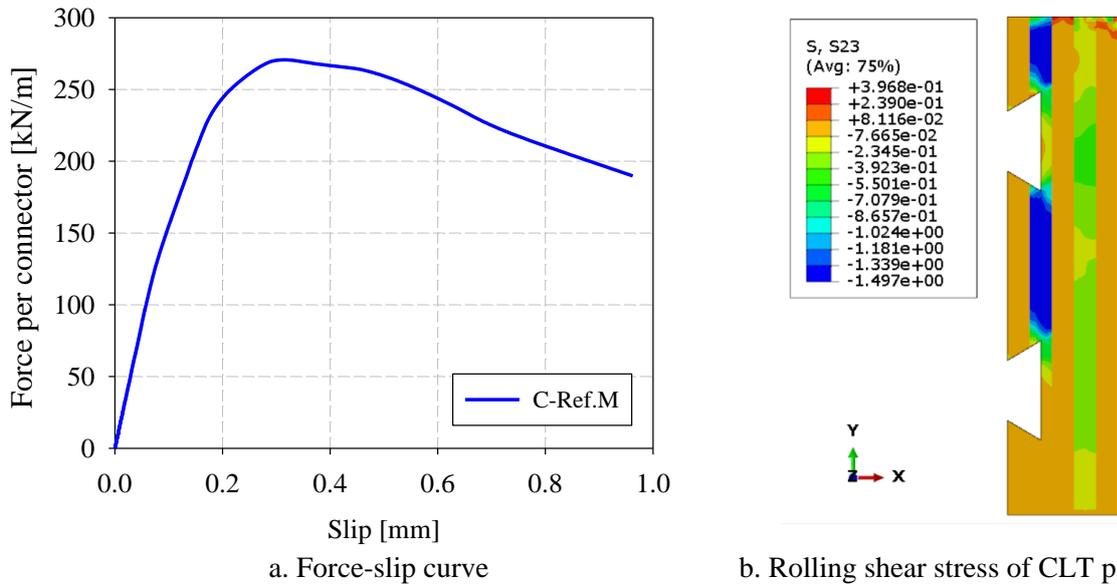
Figure 29: Force-slip curve and rolling shear stress obtained in the FE model of the case C-Ref.M.
