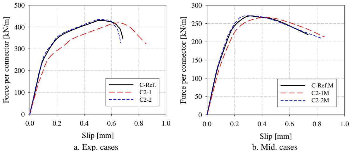
Figure 38: Force-slip curves of case series C2.
