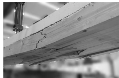
c. Bending tension failure
