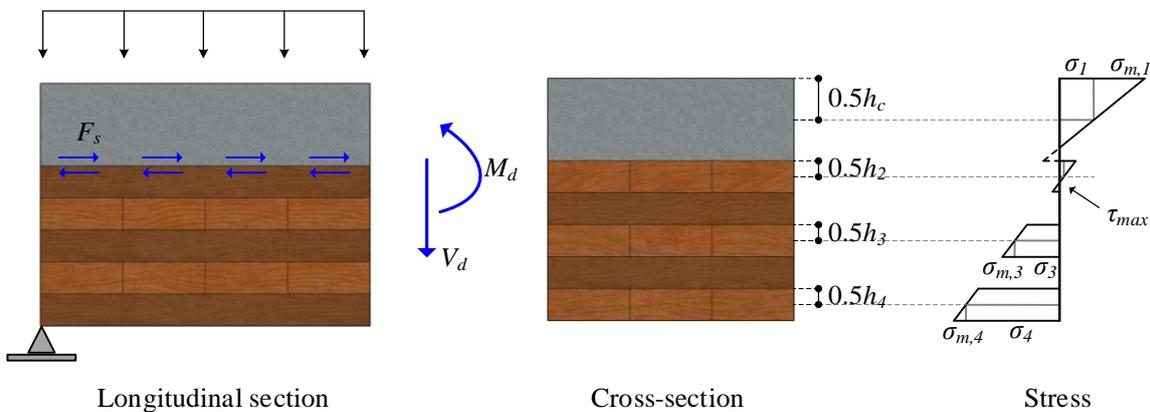
Figure 6: Stress distribution in cross-section of composite floors.
