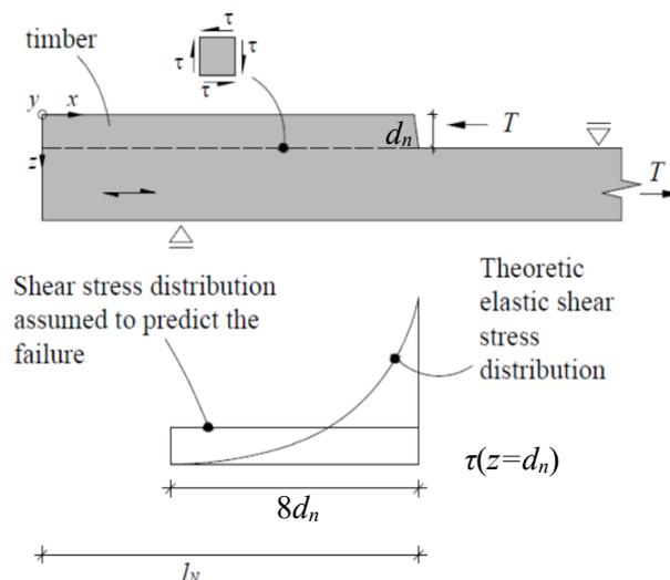
Figure 28: Shear stress distribution in the timber [92].
