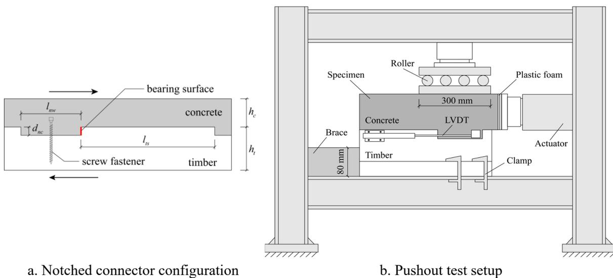
Figure 21: Notched connector and pushout test setup [19].
