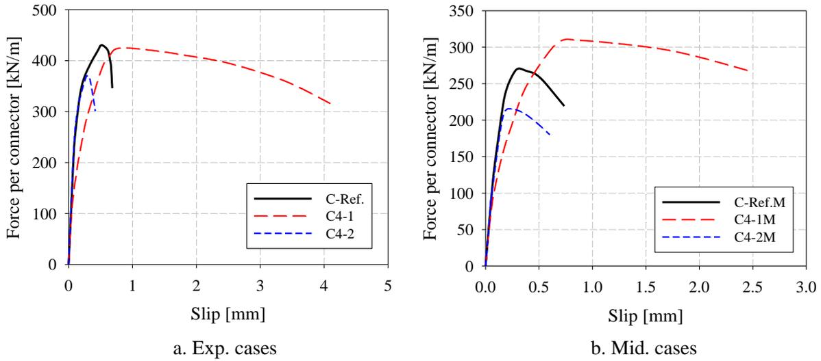
Figure 41: Force-slip curves of case series C4.
