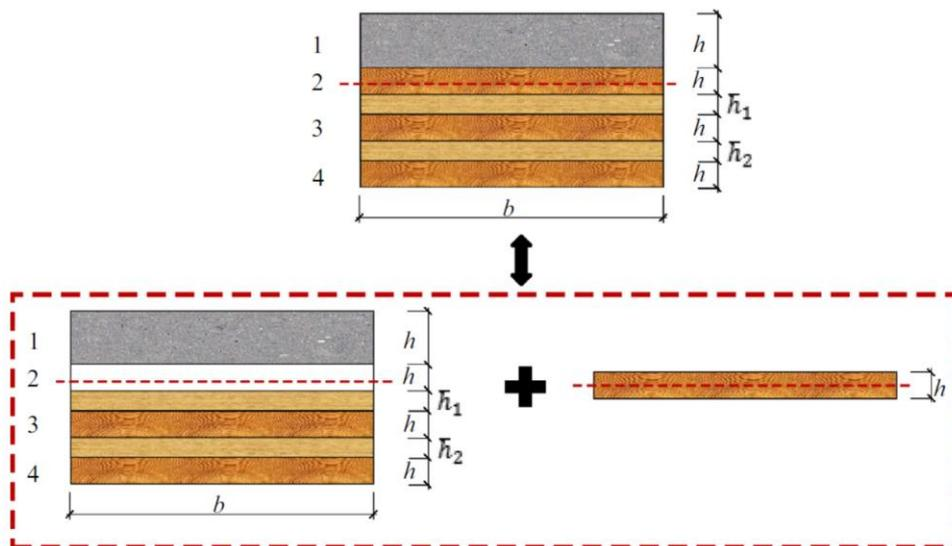
Figure 25: Calculation of 5-layer CLT-concrete composite floor [97].
