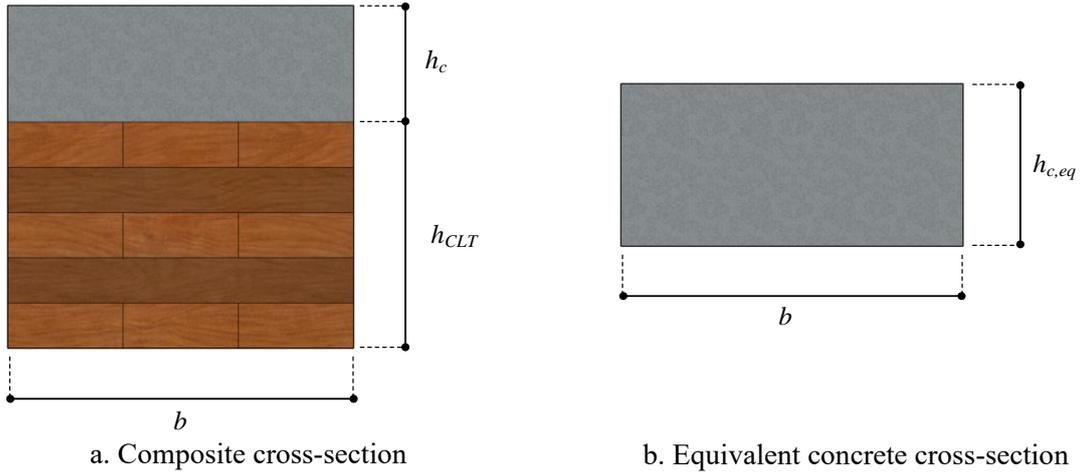
Figure 31: Composite section and equivalent concrete section.
