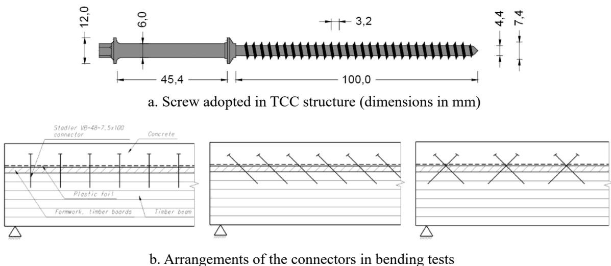
Figure 15: TCC connector and its arrangements in bending tests described by Meierhofer [83].
