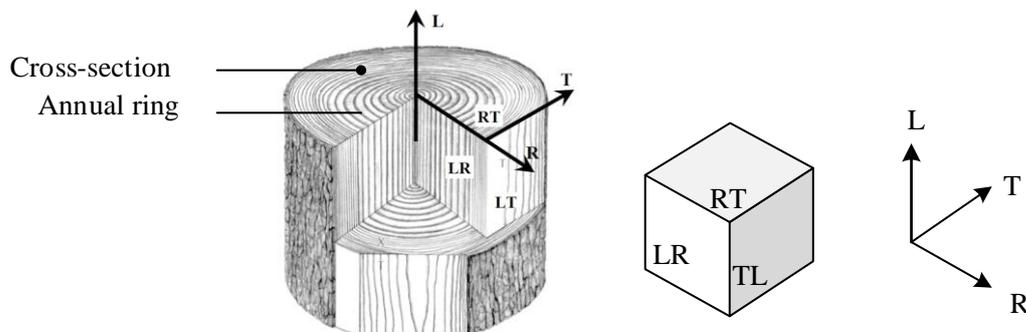
Figure 7: Structural directions of timber in the tangential (T), radial (R), and longitudinal (L) directions [48].
