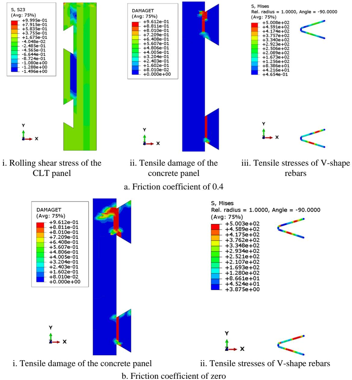
Figure 33: Failure mode and stress of components in FE models under various friction coefficients at a maximum load level.
