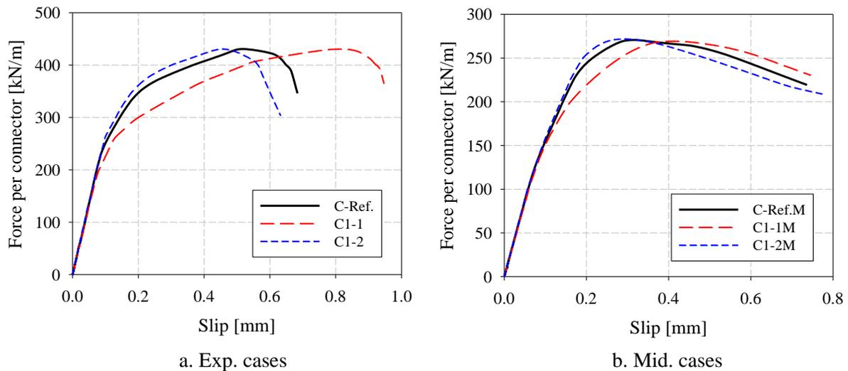
Figure 36: Force-slip curves of case series C1.
