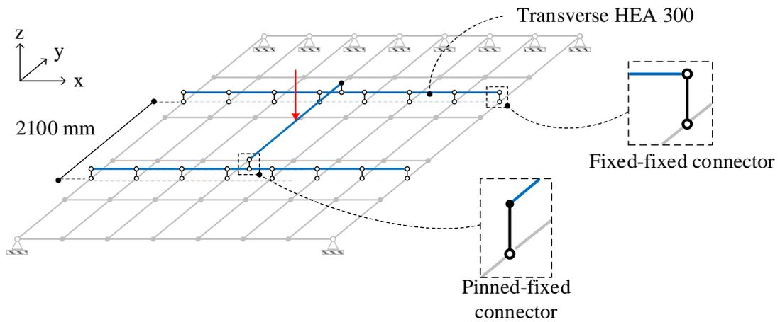
c. Loading system in beam grid model
