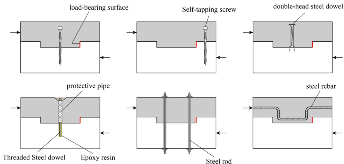
Figure 19: Reinforcing techniques in notched connectors [16].
