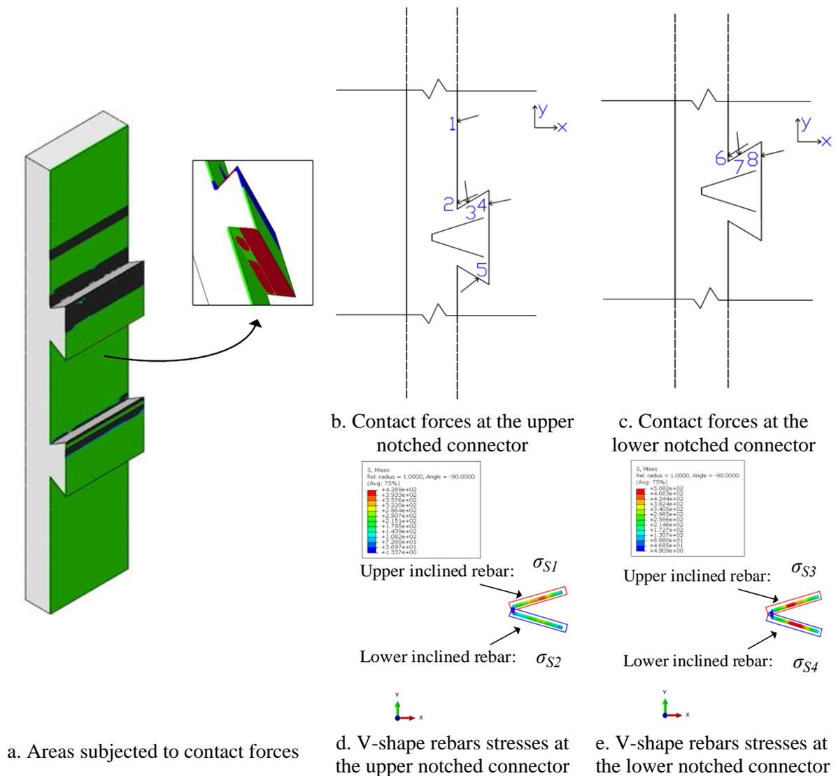
a. Areas subjected to contact forces      d. V-shape rebars stresses at the upper notched connector      e. V-shape rebars stresses at the lower notched connector
