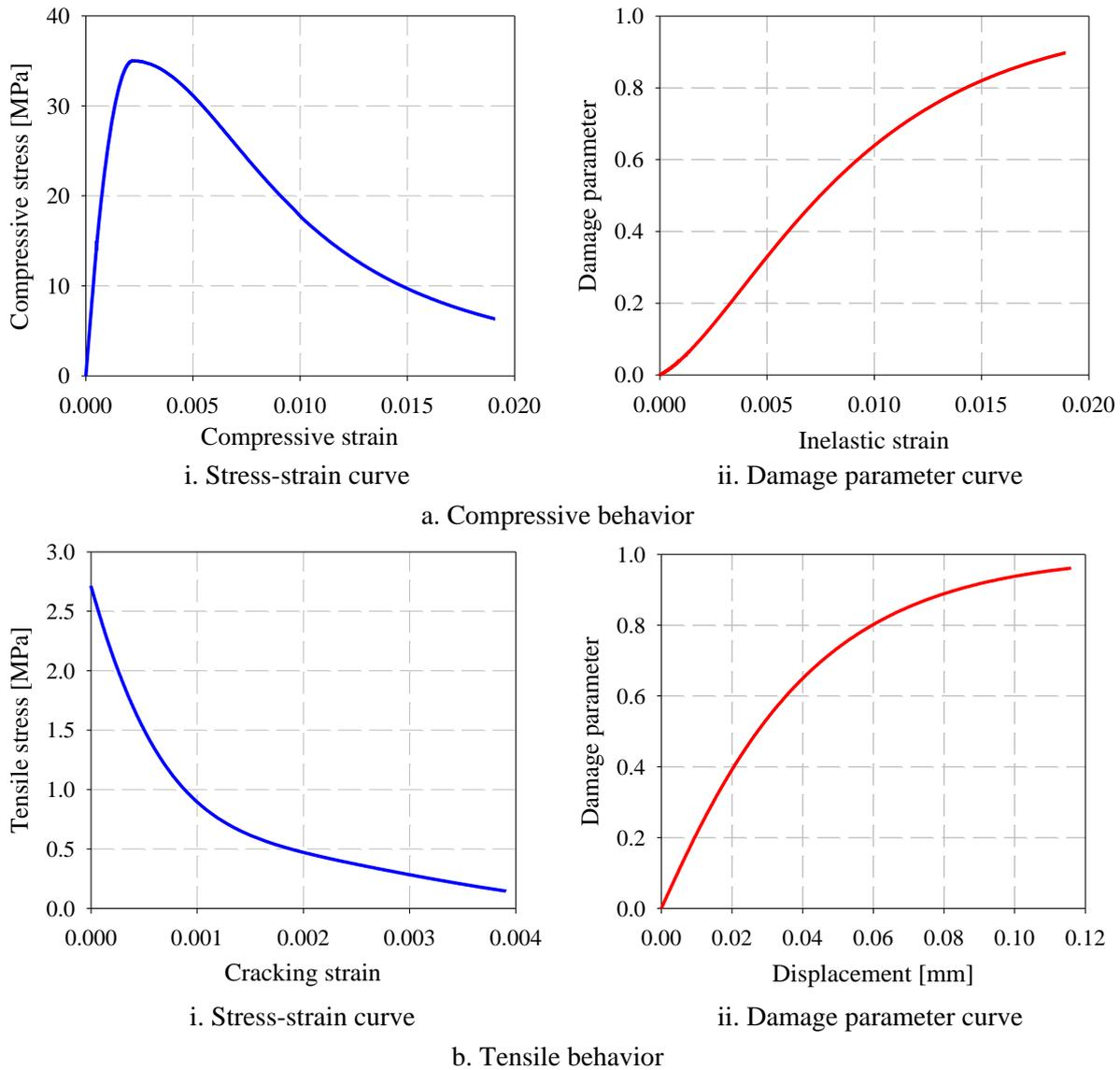
Figure 16: Constitutive concrete model in the numerical simulation.
