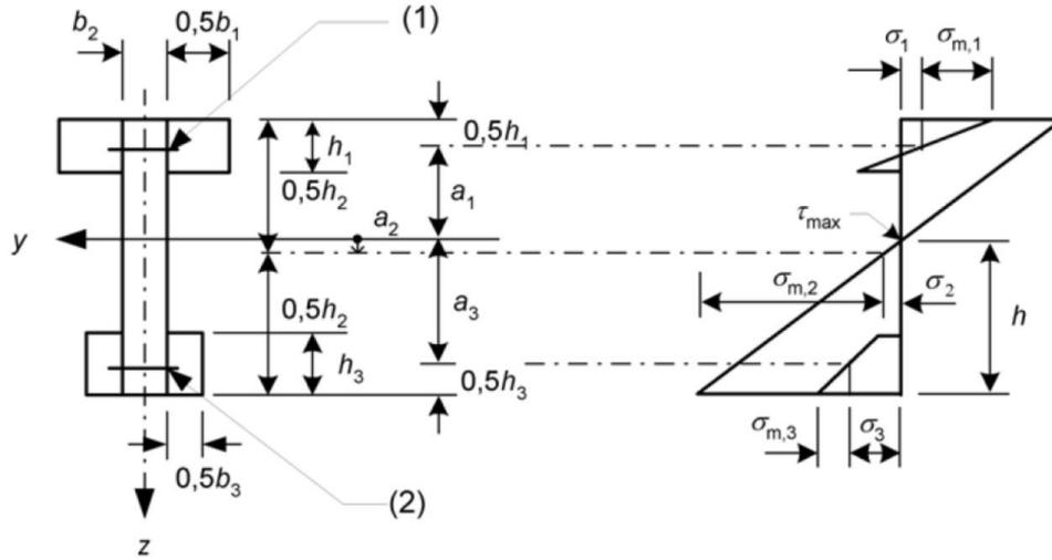
Figure 24: Cross-section and stress distribution of a composite section described in Eurocode 5 [62].
