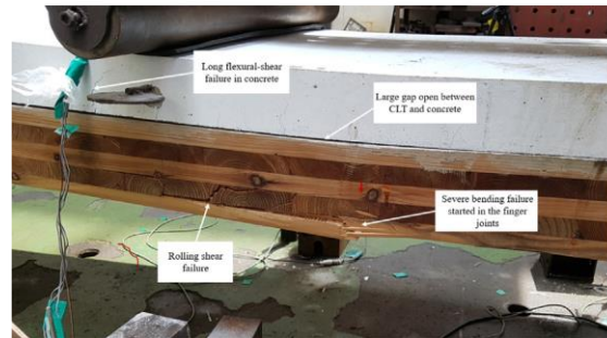
c. Typical failure mode in flexural tests
