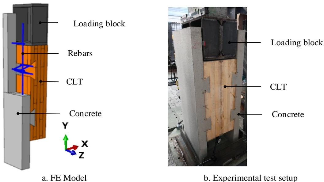
Figure 14 : Configuration of pushout test setup in FE model and experimental test.
