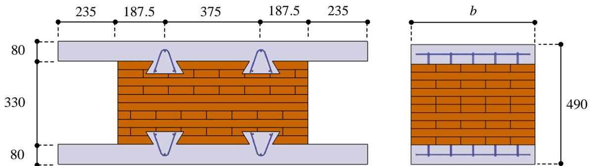
Figure 3: Dimension of pushout specimens (unit in mm).
