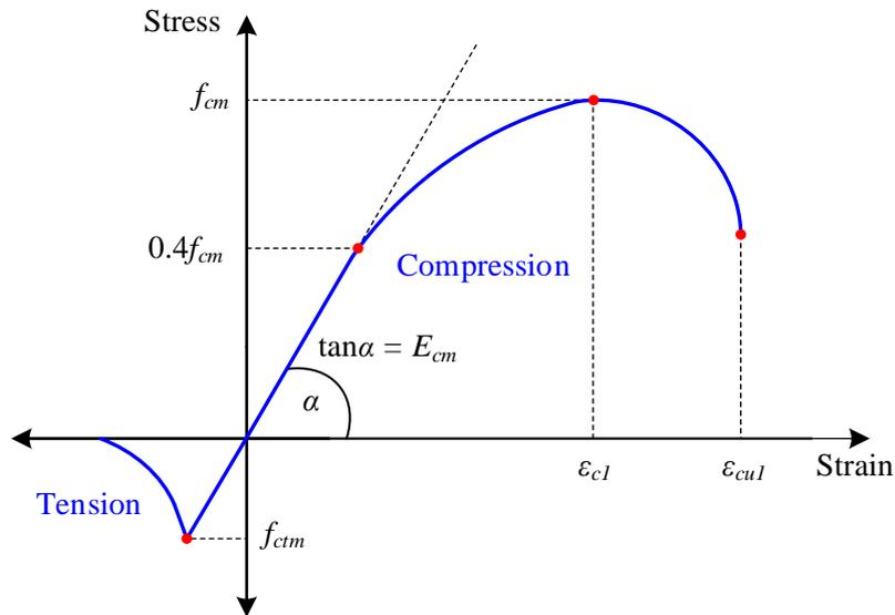
Figure 5: Typical stress-strain relationship of concrete in uniaxial compression and tension [42].
