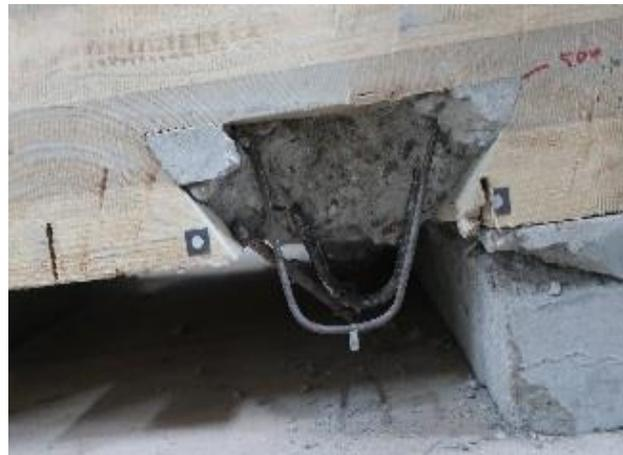
Figure 10: Steel rebars in the concrete notched connectors after collapse (concrete was removed by a jackhammer).
