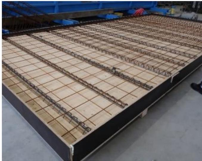
Figure 2: Photo of the specimen before the casting of concrete.
