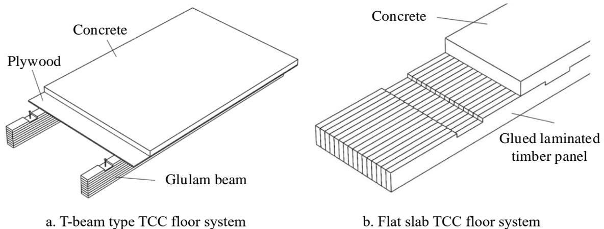
Figure 2: Two types of TCC floor systems [16].
