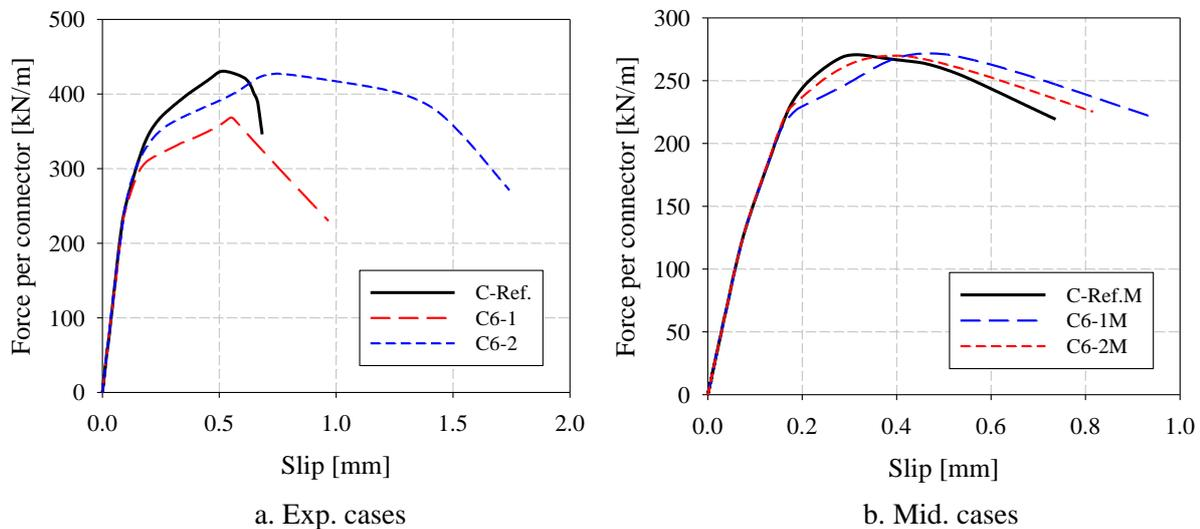
Figure 46: Force-slip curves of case series C6.
