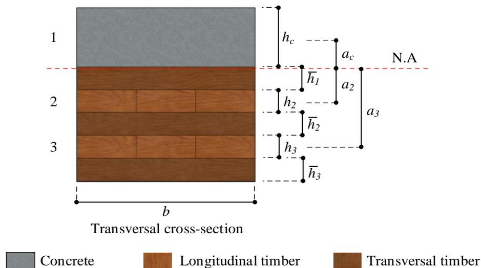
Figure 1: Cross-section of composite floor in transversal direction.
