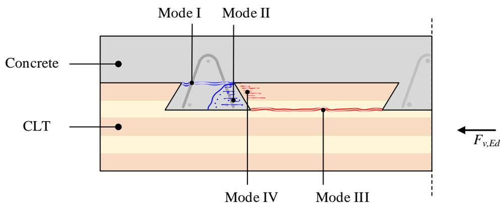
Figure 3: Four possible failure modes for notched connector.
