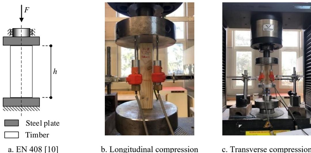
Figure 7: Test setup for timber compression tests.
