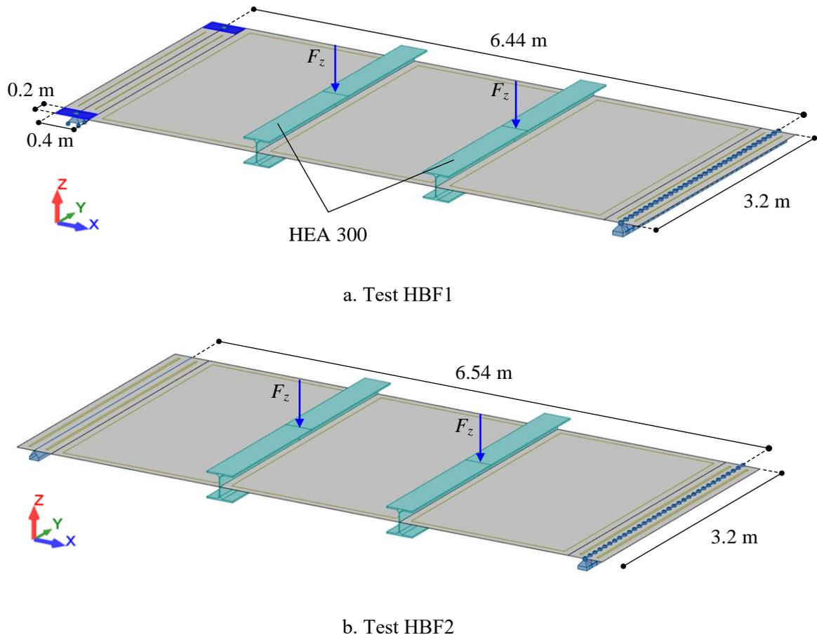
Figure 33: Orthotropic plate models of flexural tests.
