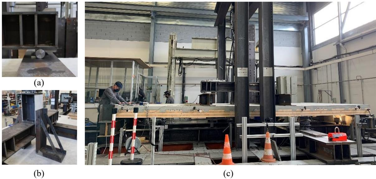
Figure 6: Photo of the flexural test setup (HBF2).
