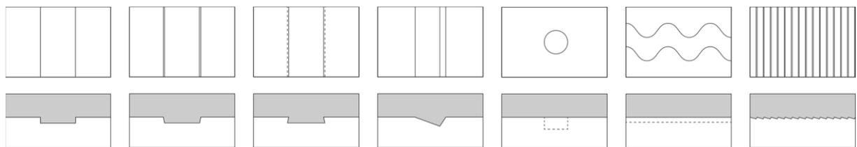
Figure 18: Different shapes of notched connectors [16].
