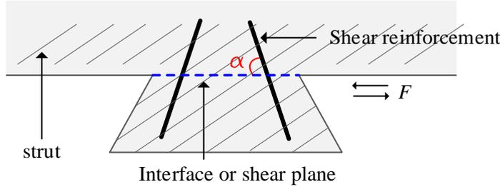
Figure 50: Assumptions of the notched connector as the concrete cast at different time.
