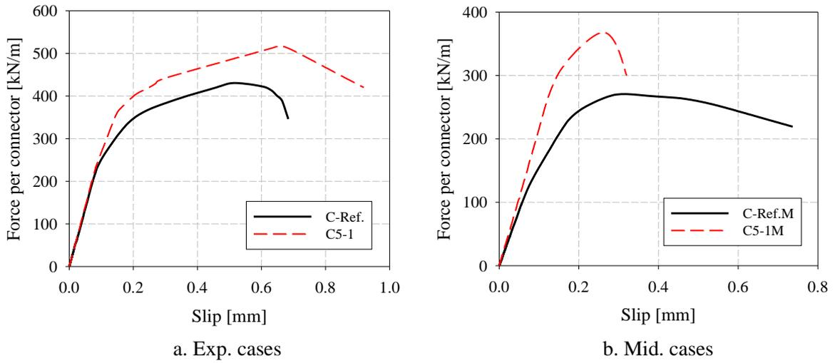
Figure 44: Force-slip curves of case series C5.
