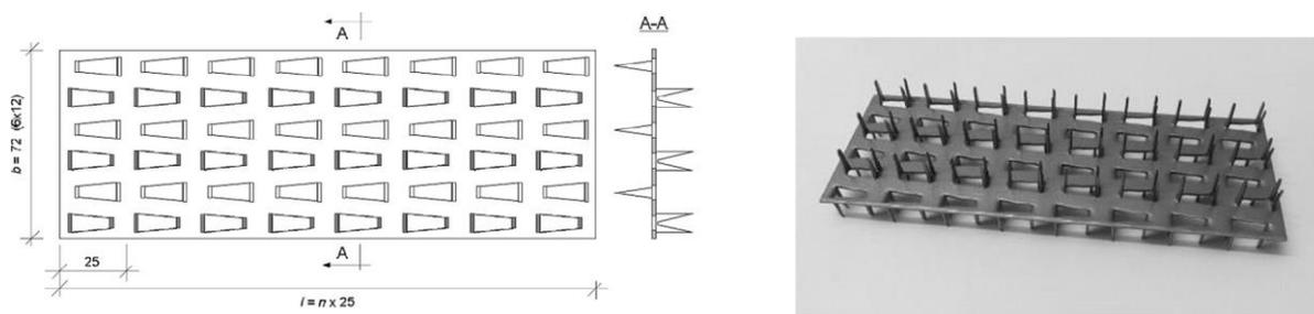
Figure 16: Nail plates as the connection system in TCC structure [87].
