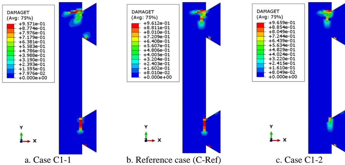
Figure 37: Tensile damage of the concrete panel in case series C1 at the maximum load level.
