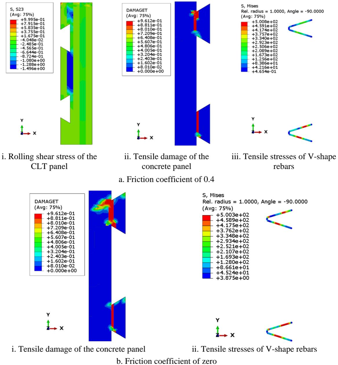
Figure 33: Failure mode and stress of components in FE models under various friction coefficients at a maximum load level.
