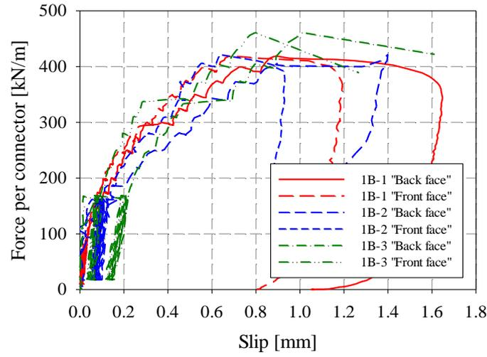
a. Force per connector versus slips
