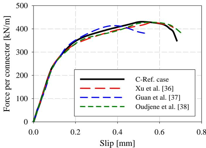
Figure 31: Slip-force curves for cases with different values of Poisson ratios.
