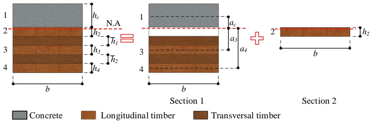
Figure 1: Computation of 5-layer CLT-concrete slabs.
