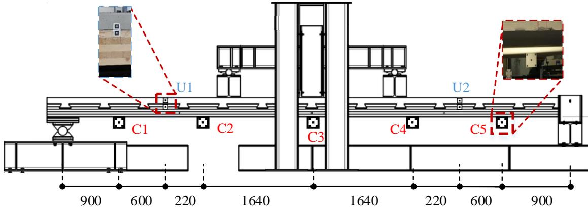
Figure 11: Measurements by digital image correlation (DIC) in flexural tests (unit in mm).
