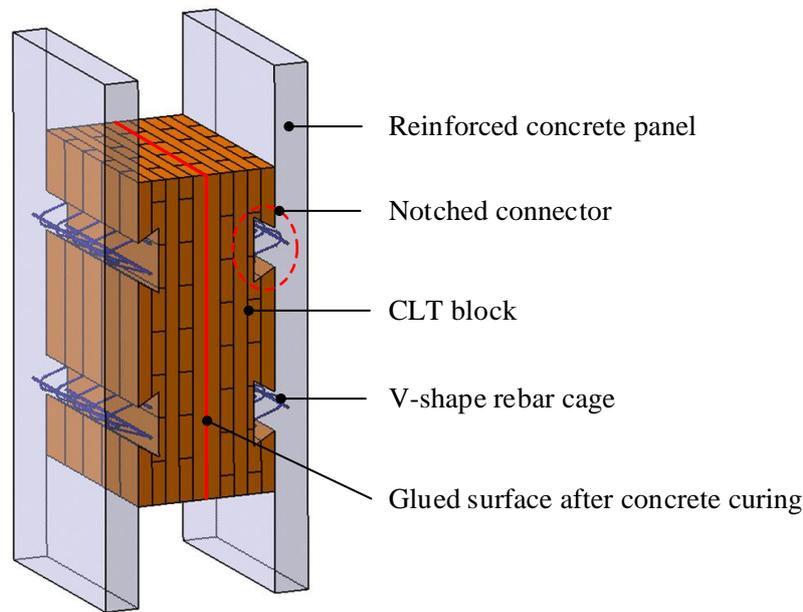
Figure 2: Description of pushout specimens.
