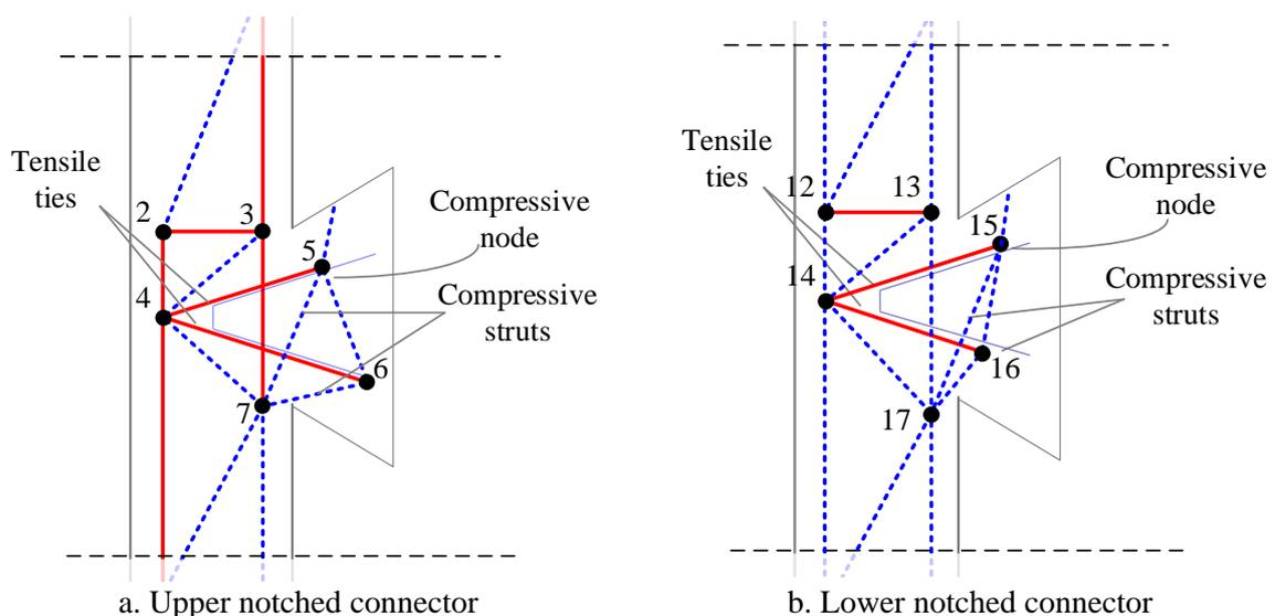
Figure 57: Compressive node, compressive strut, and tensile tie of the strut-and-tie model subjected to possible failure mechanisms based on the study of Michelfelder [49].
