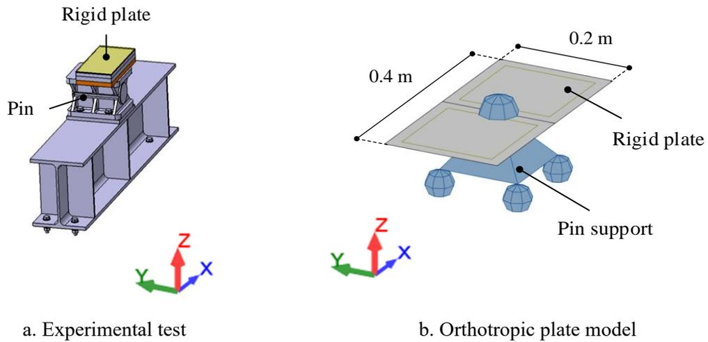
Figure 34: Model of the point support in test HBF1.
