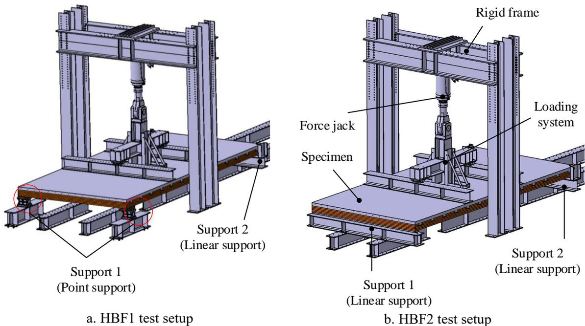
Figure 3: Flexural test setups.
