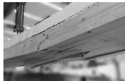
c. Bending tension failure
