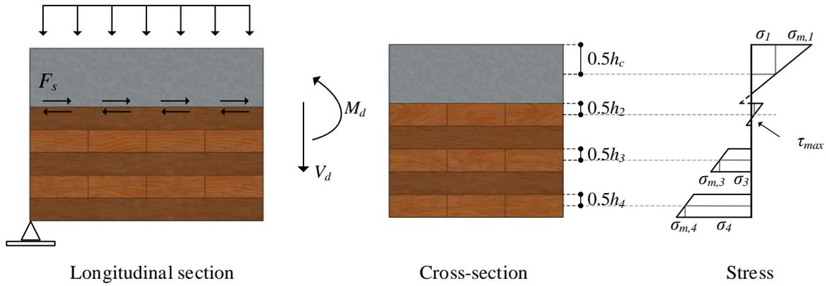
Figure 26: Stress distribution in cross-section.
