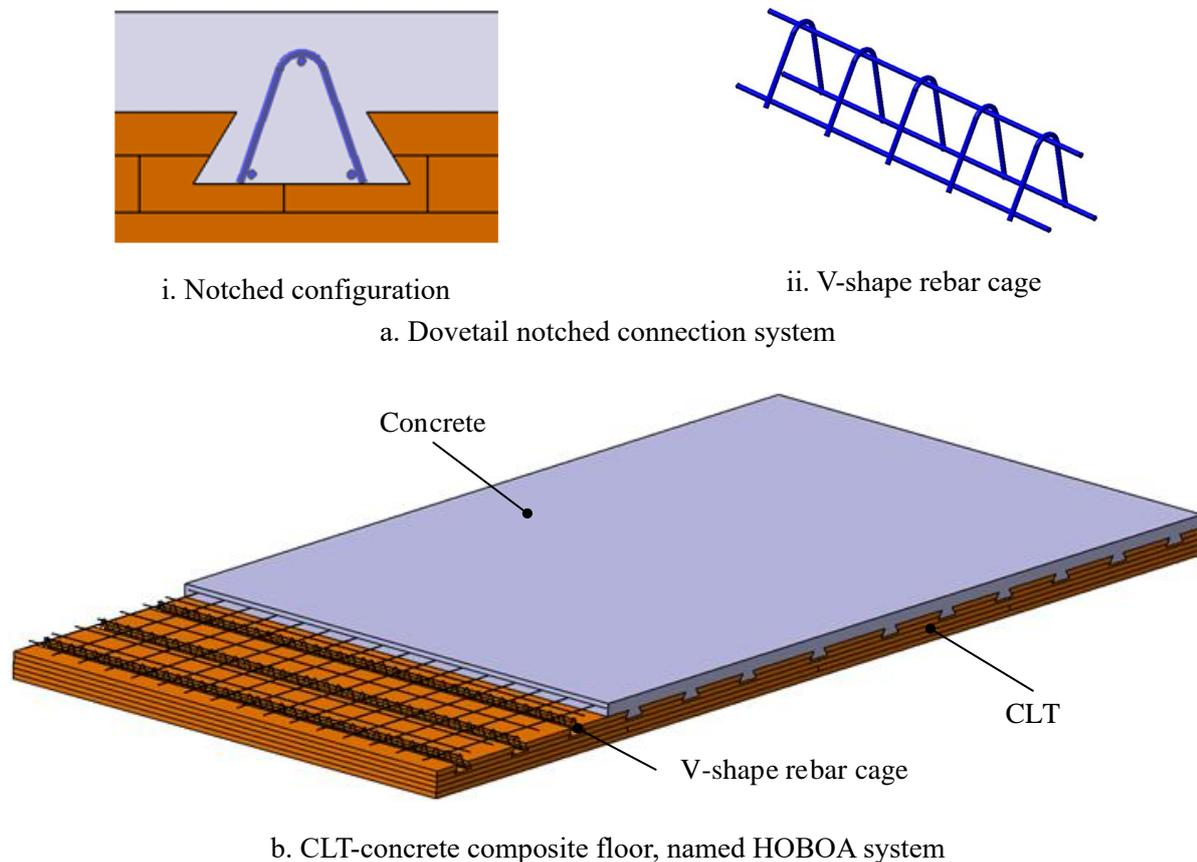
Figure 1: CLT-concrete composite floor, named HOBOA system with connection made by notches.
