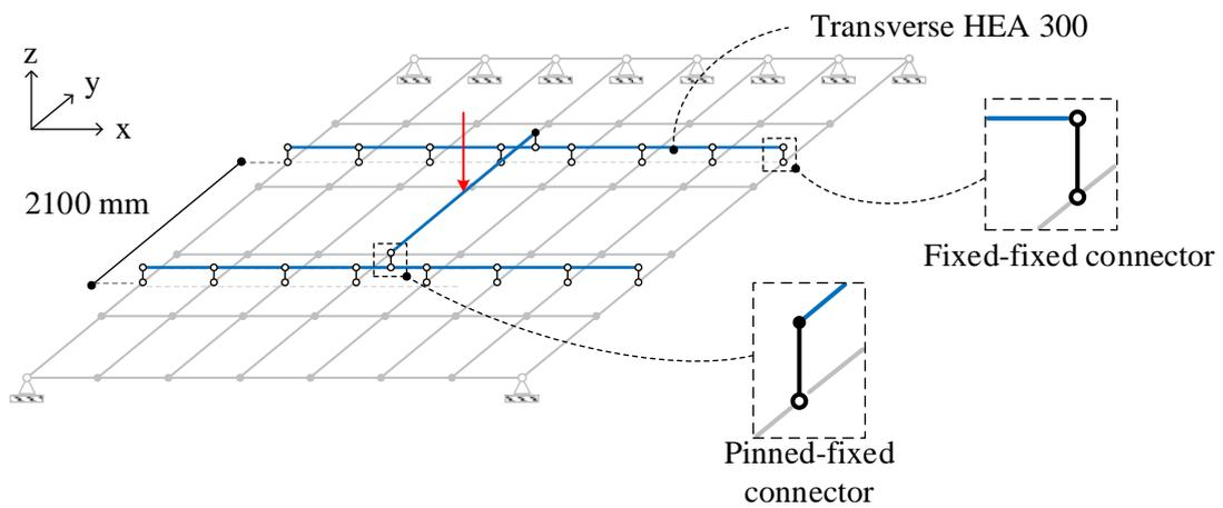
c. Loading system in beam grid model
