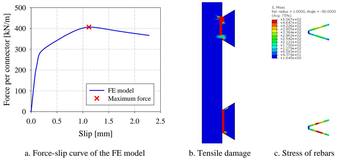
a. Force-slip curve of the FE model      b. Tensile damage      c. Stress of rebars
