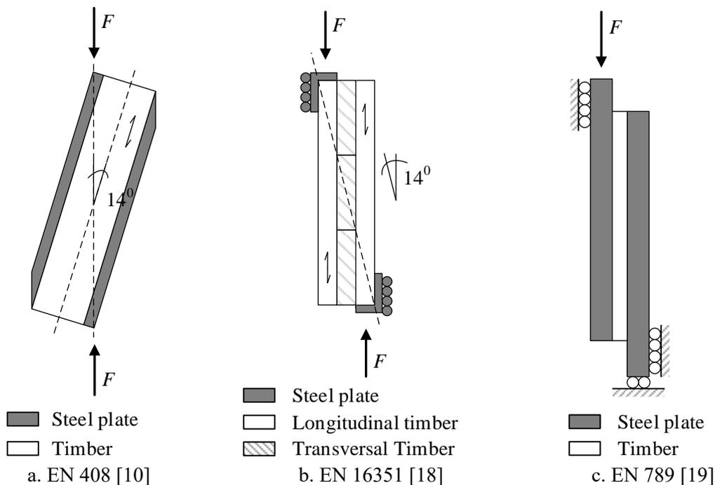
Figure 8: Direct shear test setups.
