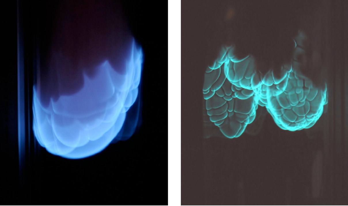
Figure 2.10: Cellular patterns on flames propagating in a tube under atmospheric conditions. Left: \text{CH}_4 -air ( \Phi = 1.3 ). Right: \text{C}_3\text{H}_8 -air ( \Phi = 1.4 ). Taken from Quinard et al. [104].
