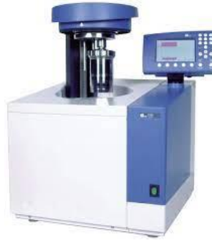
Figure IV. 5: Bombe calorimétrique IKA C2000 Calorimeter Basic
