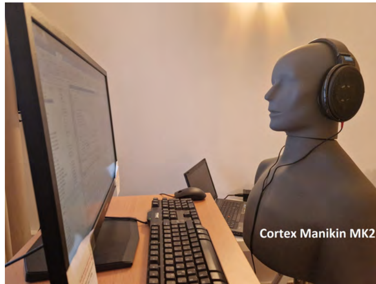
Figure 6.1: The Cortex Manikin MK2 used before the psychoacoustic test. Before conducting the test, it was necessary to measure the sound pressure level, expected to be heard by participants, by means of the Cortex Manikin MK2
