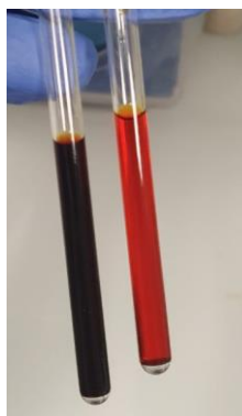
Figure 5.4.1 Photo of a tube with L1PF_6 in AcN-d_3 (red) and of L1PF_6+t-butOK in AcN-d_3 (dark-red).
