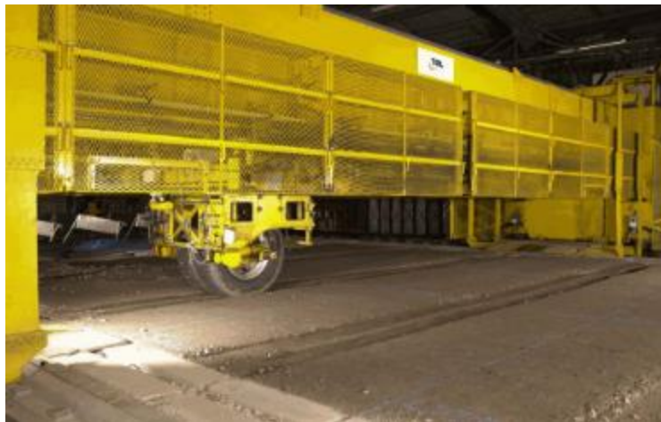
Figure 2-22: Pavement test facility (Watts et al., 2004)
