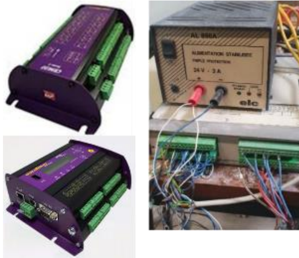
Figure 3-27: Data Taker setup, and Scaime setup with the external generator of the laser sensors.
