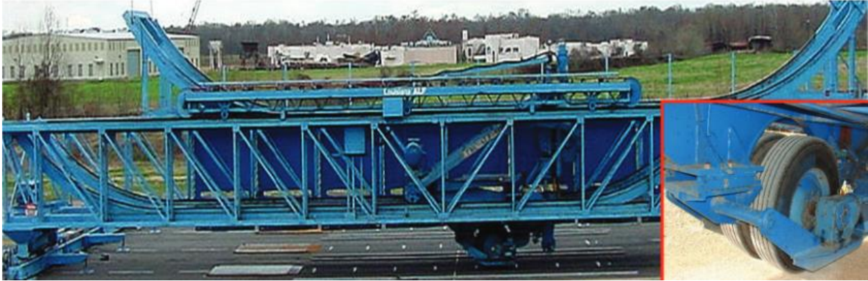
Figure 2-20: ALF with insertion of dual-wheel assembly
