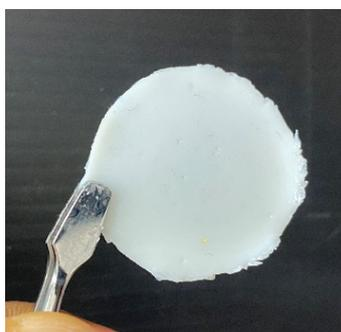
**Figure 7.** Exemplary pictures of as-fabricated SPE before vacuum drying. In this photo, the sample is  $S\text{-SPE}_{15-92\%}$  ( $\varnothing$  30 mm, thickness  $\approx 500 \mu\text{m}$ ).
