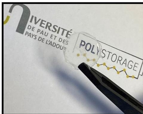
**Figure 24:** Exemplary pictures of self-standing transparent films ( $\varnothing$  16 mm,  $L= 100 \mu\text{m}$ ) derived from block copolymer electrolyte  $sc\text{-(A}_{0.62}\text{)}_{0.80}\text{B}_{0.20}$ .
