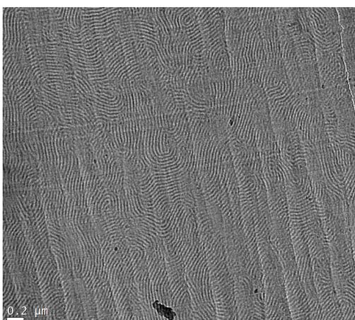
**Figure S30.** TEM images for annealed linear comb-like BCPE:  $lc-(A_{0.59})_{0.71}B_{0.29}$ ,  $\phi_c = 0.29$
