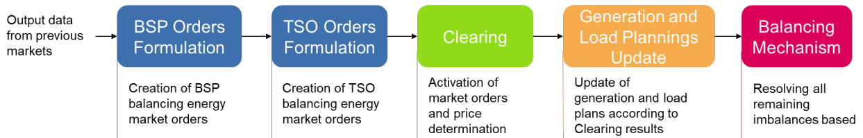
Figure 2.3: Macro overview of ATLAS balancing stage modules
