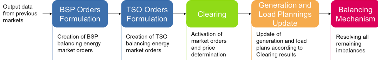
Figure 3.12: Macro overview of ATLAS balancing stage modules
