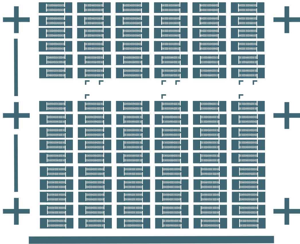
Figure 3.6: Lithography mask design for trumpets. Each subfield consist of 32 devices with identical top diameter.
