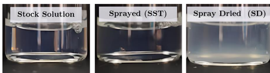
Figure 4.8. Pictures from formulation F1.100 a) Stock solution b) sprayed solution (from SST, non-dried), c) reconstituted solution from spray-dried powder
