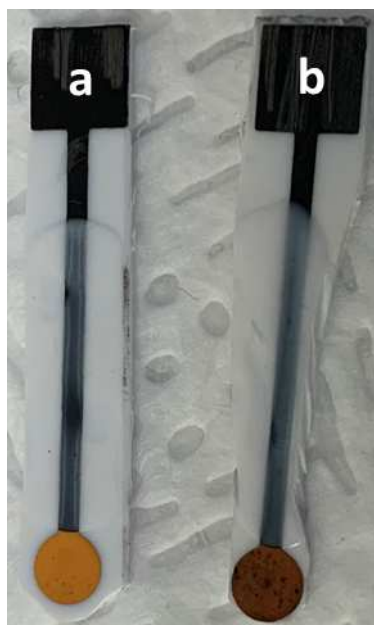
Figure III-4. Images of (a) well-homogenized deposition of gold nanoparticles, yielding a soft yellow surface, and (b) poor deposition resulting in black surfaces.
