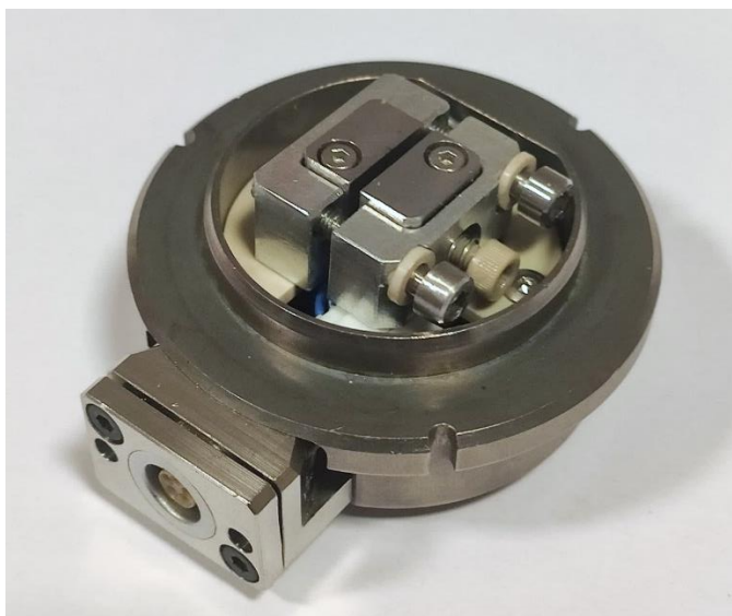
Figure 97: Improved operando cell with two stainless steel screws to achieve higher stack pressure.
