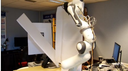
(a) Initial configuration where camera looks at target point that is placed in between two obstacles
