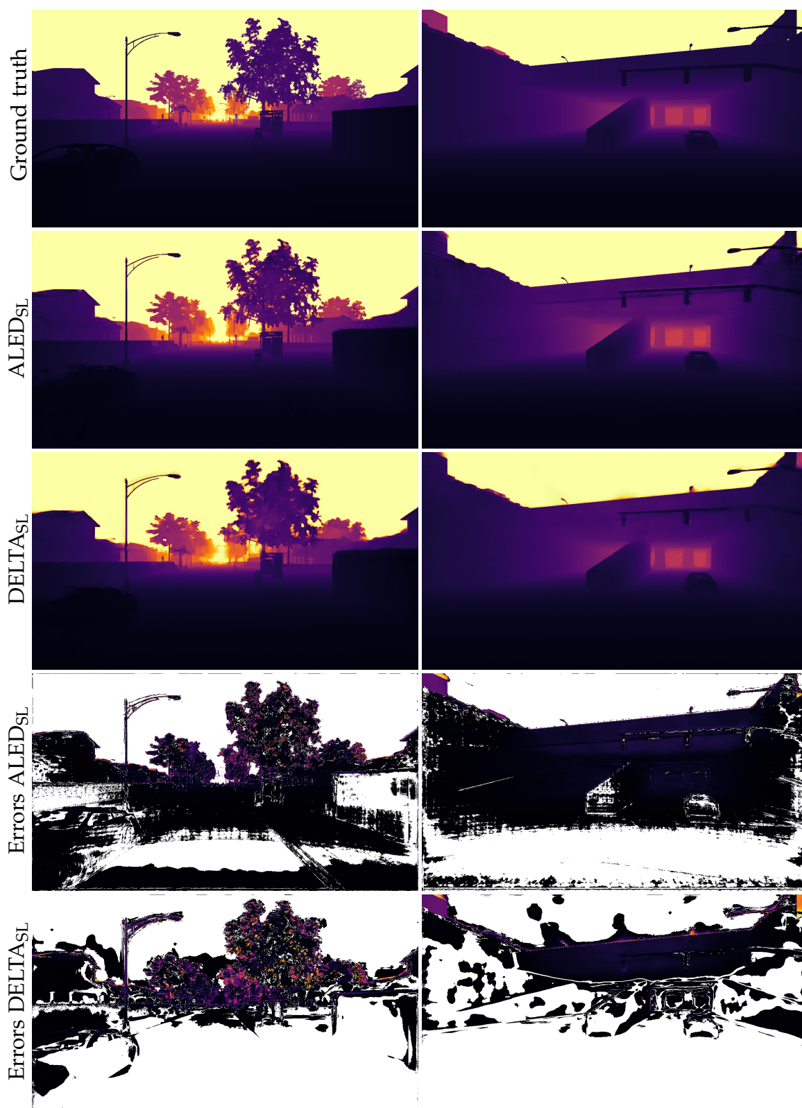
Figure 5.6 – Results on the Town01_08 (left) and Town03_19 (right) sequences of our SLED dataset, for the “before” depth map D_{bf} . From top to bottom: ground truth depth map; result from ALED sL ; result from DELTA sL ; error maps of both methods, where pixels with an error inferior to 0.5m are in white.
