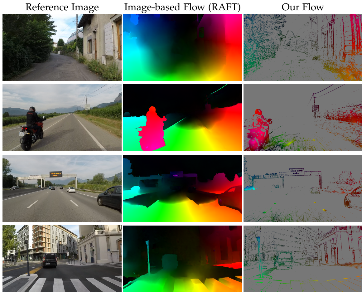
Figure 3.7 – Qualitative results on the 20-minute-long driving sequence. Extracts used, from top to bottom: a village street, a motorcycle overtaking, a highway, and an intersection. Best viewed in color.
