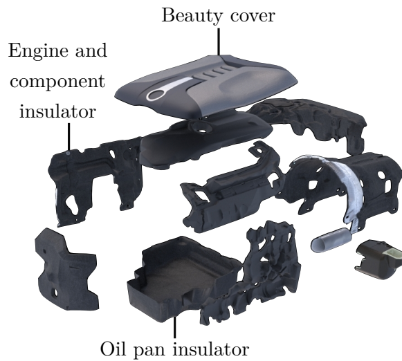
Figure 6. Possible encapsulation components of a car engine using poroelastic screens [28].
