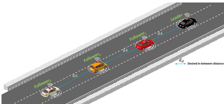
**Figure 1.16.** Cooperative adaptive cruise control: platooning navigation
