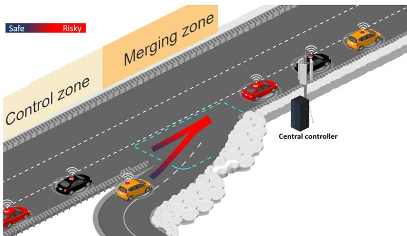
**Figure 2.22.** Centralized collaborative on-ramp merging on highway
