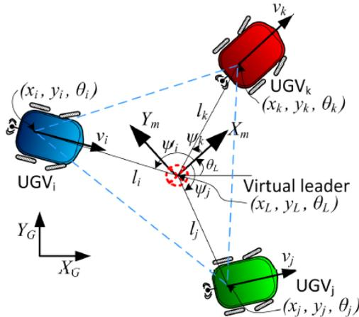
**Figure 2.10.** Virtual structure formation modeling approach [238]
