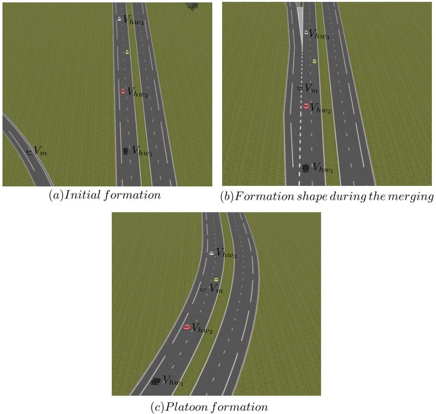
**Figure 4.14.** Snapshots of the evolution of the formation shape during the on-ramp merging scenario obtained with the help of SCANer studio ([Simulation video: https://youtu.be/3gDSq5L3m-c](https://youtu.be/3gDSq5L3m-c))
