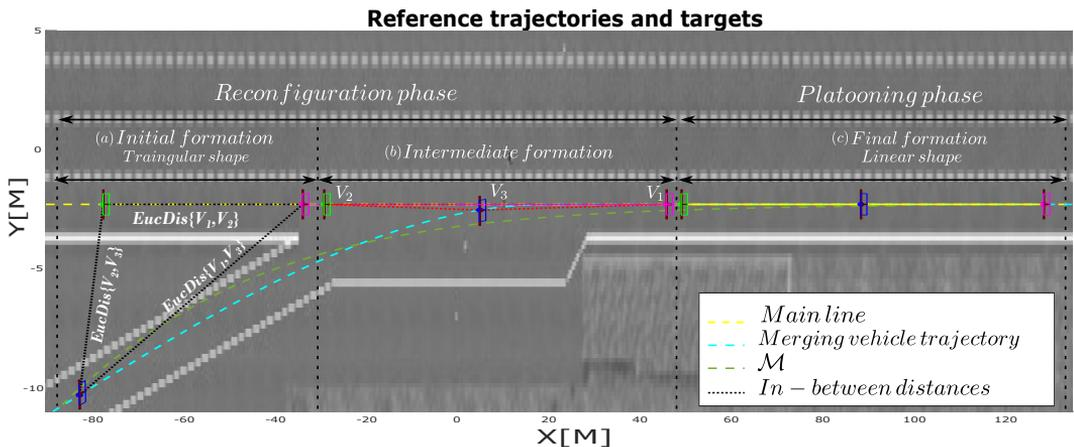
**Figure 4.5.** Evolution of the formation shape during the merging performed by the CORM framework (Simulation video: <https://youtu.be/UM2cLt74pVM>)
