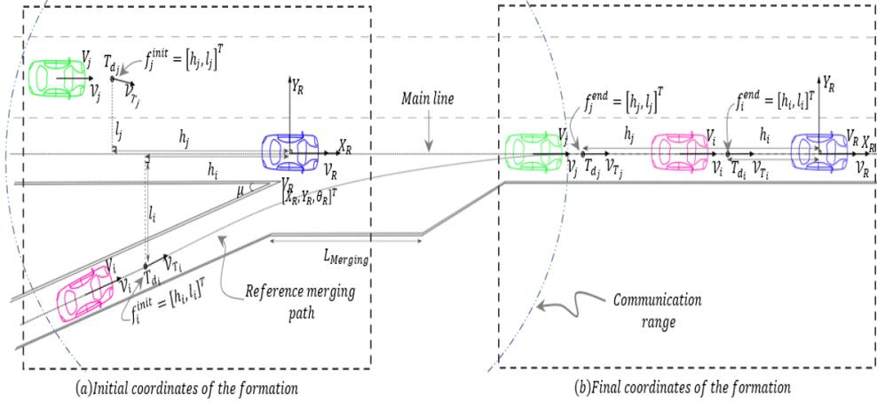
**Figure 4.1.** The virtual structure approach used to model the formation and its reconfiguration to perform the merging maneuver. (a) The initial shape of the formation and its coordinates. (b) The final shape of the formation after the merging maneuver and its desired coordinates.
