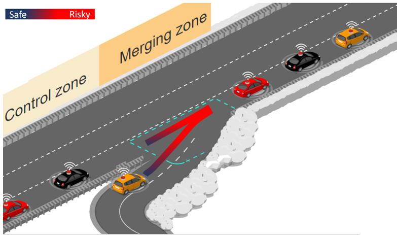
**Figure 2.23.** Decentralized collaborative on-ramp merging on highway
