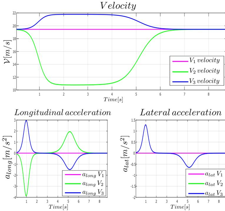
**Figure 4.7.** The vehicles' velocity and acceleration profiles
