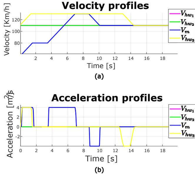
**Figure 5.12.** The vehicles' velocity and acceleration profiles
