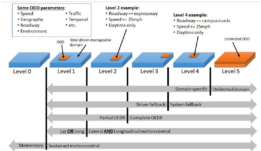
**Figure 1.2.** SAE autonomy levels ODD's [119]
