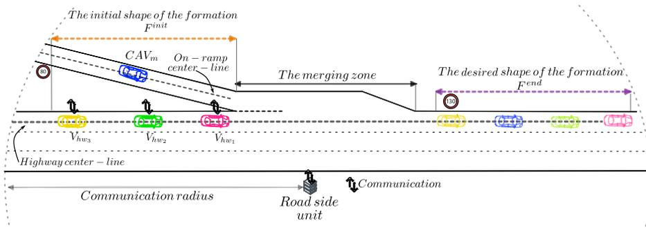
**Figure 5.9.** Scenario 1: Illustration of the on-ramp merging on highway scene. The initial shape of the formation under the communication range of the RSU is represented, along with the desired shape
