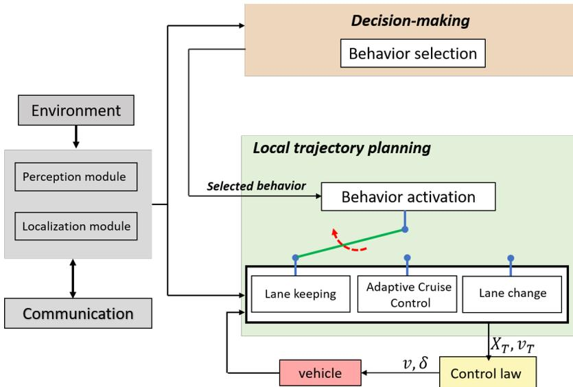
**Figure 3.1.** Multi-Controller Architecture
