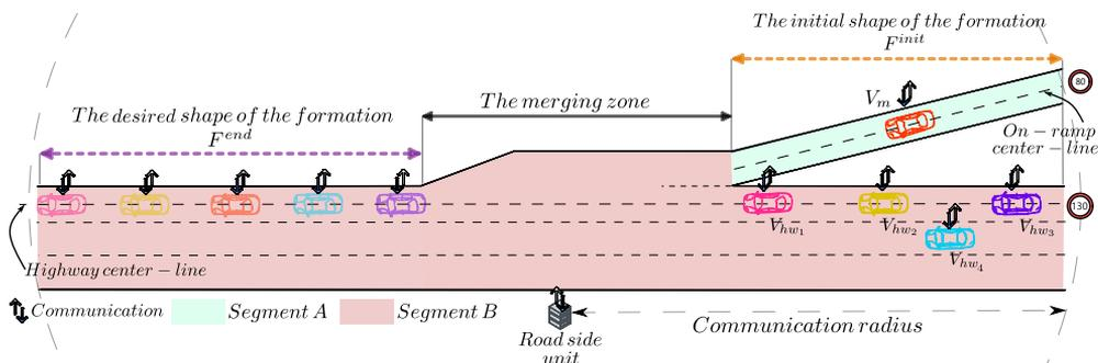
**Figure 5.13.** Scenario 2: Illustration of the on-ramp merging on highway scene. The initial shape of the formation under the communication range of the RSU is represented, along with the desired shape (Simulation video: <https://youtu.be/u0LRJbOW94M>)
