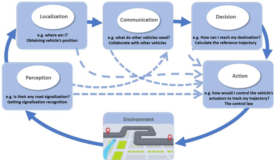
**Figure 2.1.** Reference control scheme for MVS, adapted from [238]
