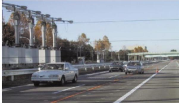
**Figure 1.6.** Platoon navigation under the DEMO 2000 project [93]
