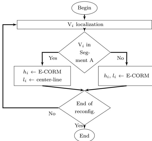
**Figure 4.9.** Coordinates selection based on the traveled segment
