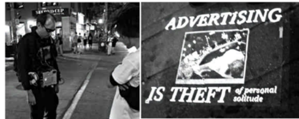
Figure 1. (a) The wearable device contains a 1 GHz P3 CPU, rendering engine, high-power mercury vapour arc lamp data projector, within a black flame-retardant Nomex uniform custom tailored to fit the wearer. Here a person can see his own image together with other computer generated material. (b) Close-up view showing the output of the high intensity data projection system.
