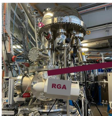
Experimental set-up to determine the gaseous radiolysis products
