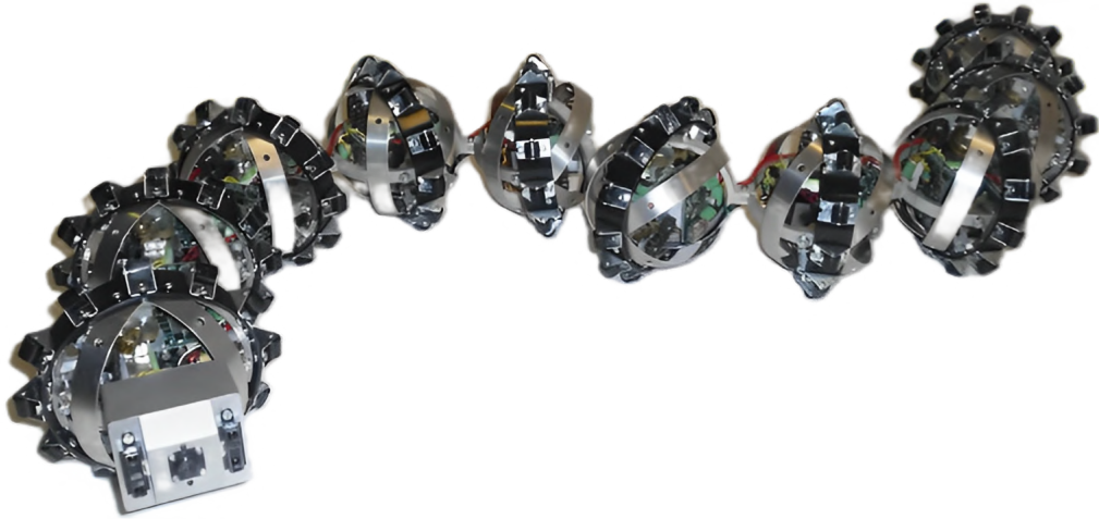
Figure 1.6: Representation of the snake robot Wheeko
