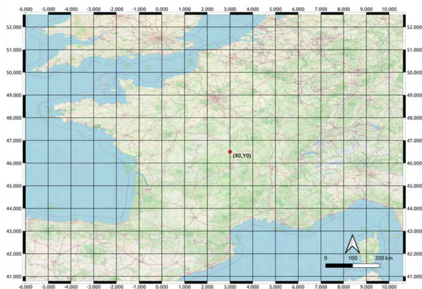
Figure 3.6: Representation of the point (X_0, Y_0) in Lambert 93 projection (background map © OpenStreetMap contributors).
