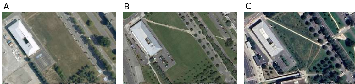
Figure 1.3: Dynamics of desire paths. Satellite images of the entrance area of the Université de Toulouse III – Paul Sabatier. (A) 2006: Absence of any discernible desire path. (B) 2013: A desire path appears after the construction of a metro and bus hub in the upper left corner. (C) 2023: The university builds an official path following the desire path. However, the introduction of Téléo, a cable car line in the lower left corner, leads to the formation of new desire paths. Credits: Google Earth.
