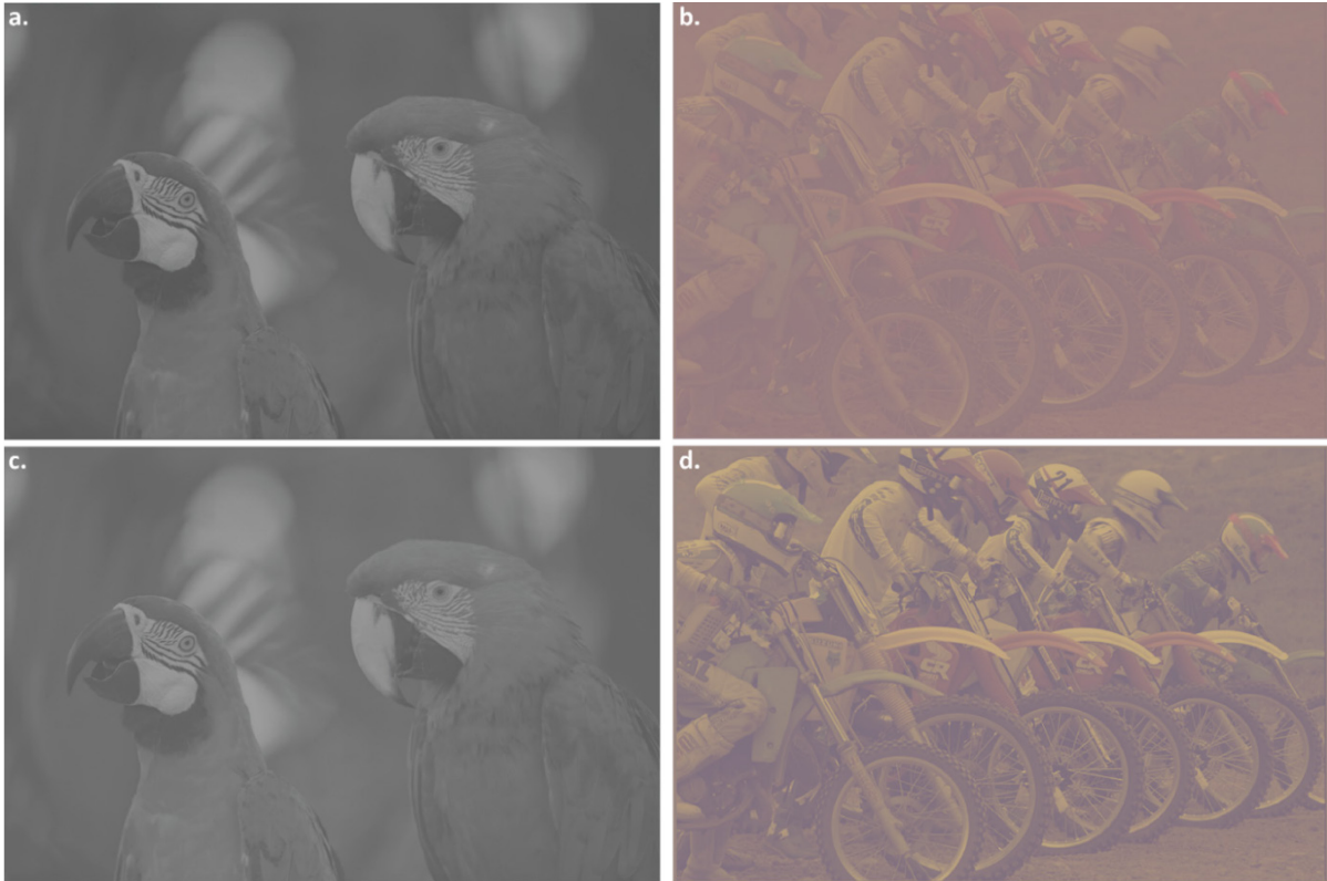
Figure 7.13 Images after multiplexed gamut mapping (a, b) without PCA (c, d) with PCA applied to the BR colors in the RG plane (b, d) transformed back to RGB for display.
