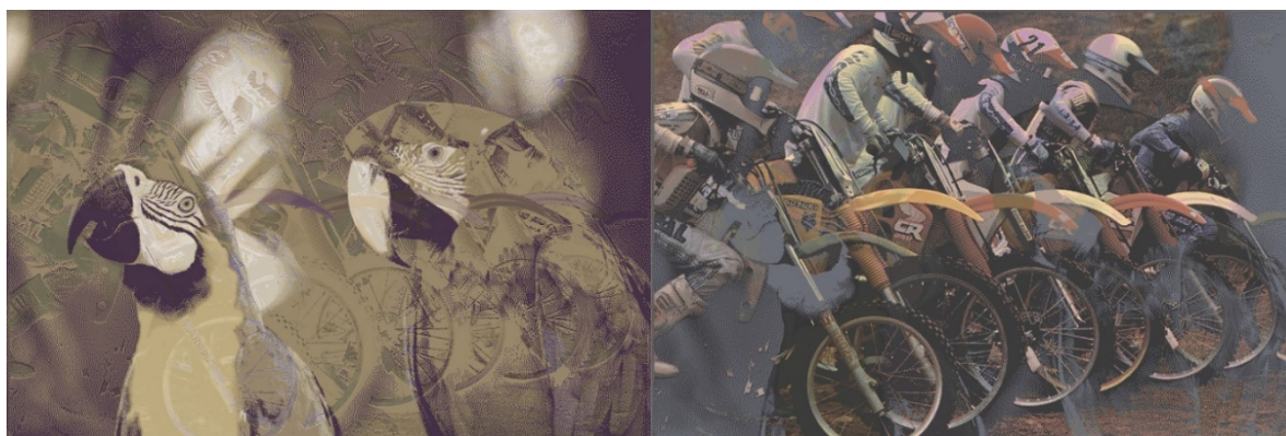
Figure 7.3 Two simulated images generated by bi-modal halftoning without gamut mapping. The color of each pixel corresponds to the colors of the selected metasurfaces in mode “transmission” (left) and mode “backside reflection” (right). Ghost images appear when colors are out of the multi-mode gamut. Original images are from the Kodak Photo CD Sampler [15] .
