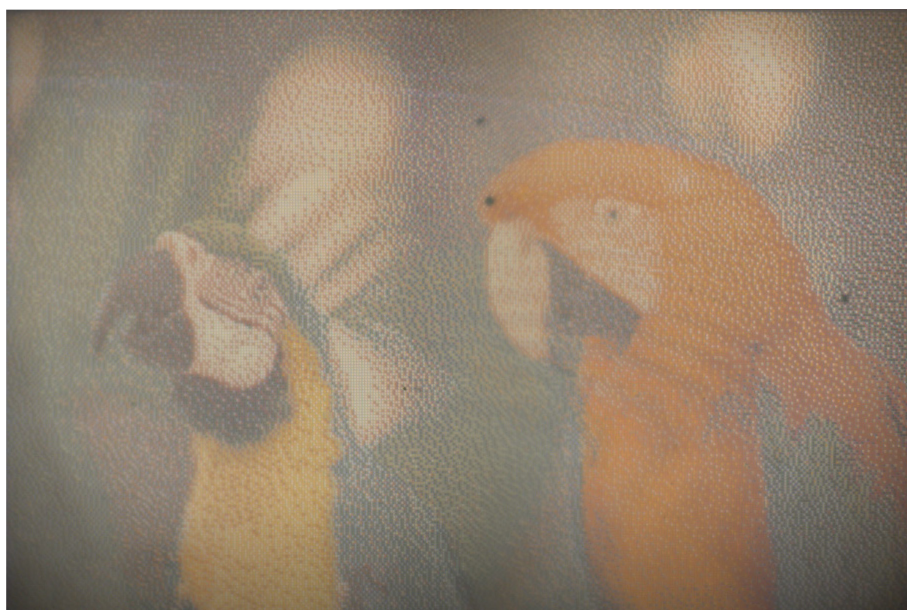
Figure 4.10 Demonstrator of a single color image printed with our laser color marking technology. The size of the printed image is 23.8 mm x 15.84 mm. Each printed pixel is a 72 \times 72 \mu\text{m}^2 square. Image taken with our imaging setup in mode "backside reflection".
