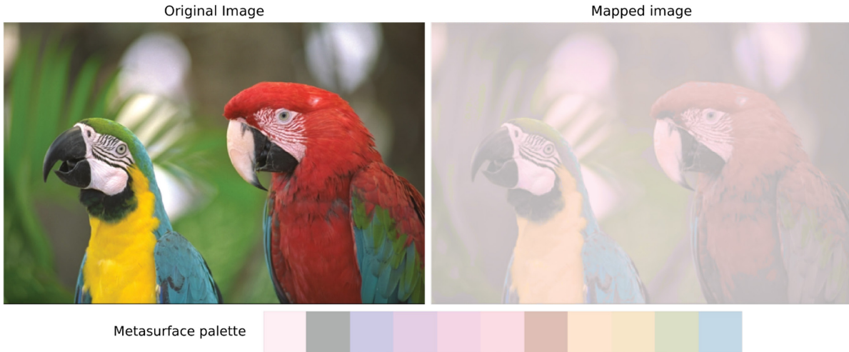
Figure 4.6 Original image and result of its gamut mapping to a palette of 11 metasurfaces in mode “backside reflection”.
