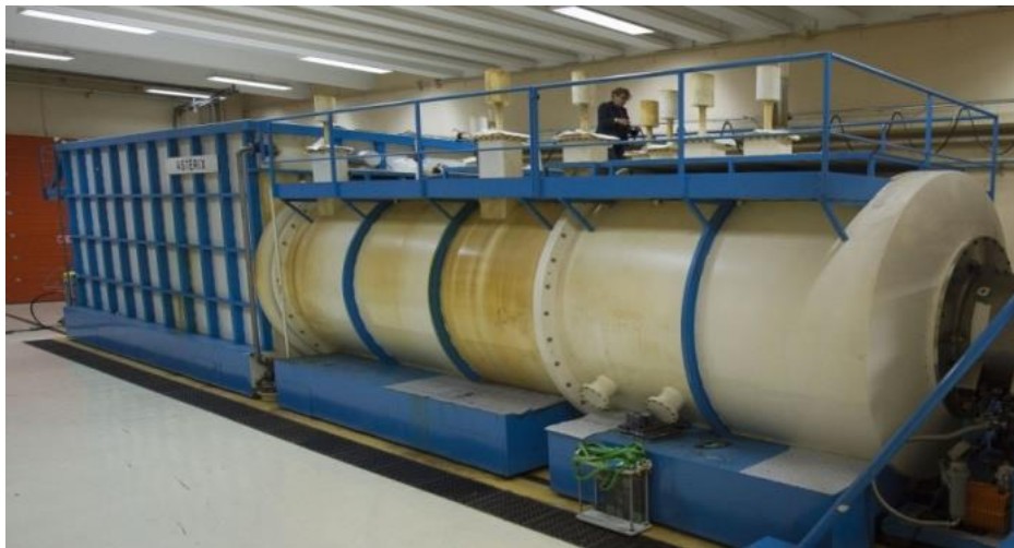
Figure 3.9. The ASTERIX pulsed X-ray generator, Centre d'Etudes de Gramat, France.
