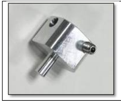
Figure 7: Sample holder used in FIB
