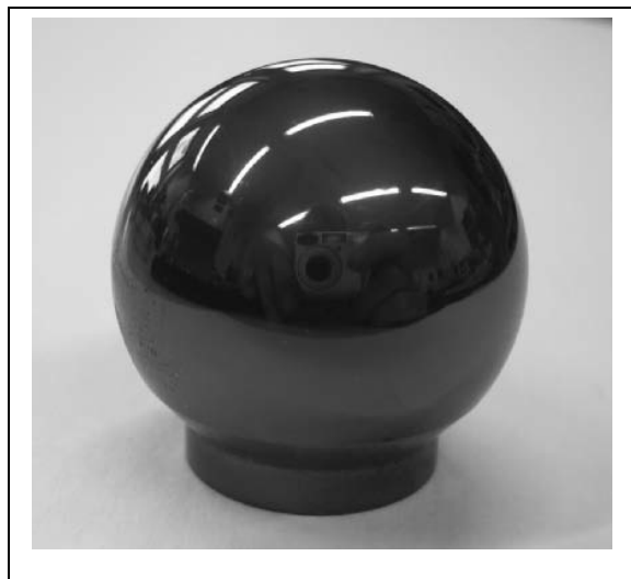
Figure 6: DLC-coated head of a hip joint [2]
