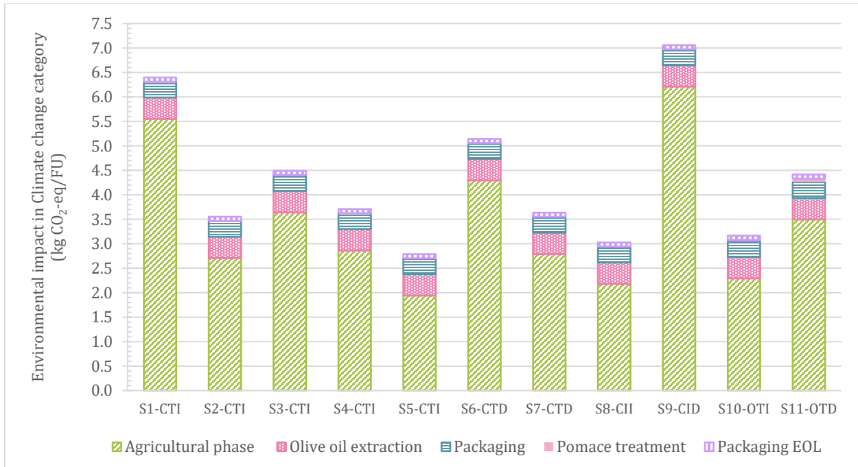
Figure II-11. Distribution of the impact of the life cycle of olive oil production in the Climate change category.
