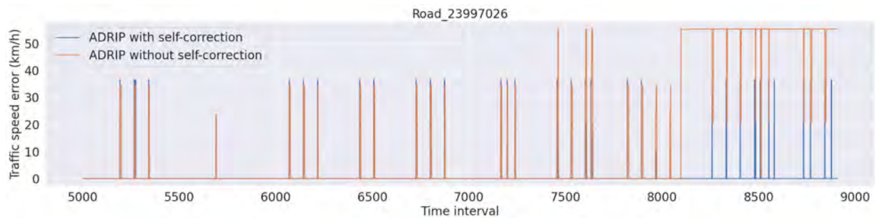
(b) Prediction errors over time on Road 23997026 (road segment with the average activation instances of the self-correction mechanism)
